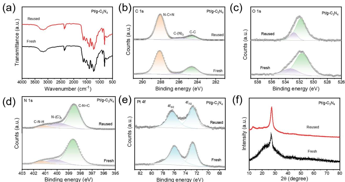
Fig. 5 The characterization of Pt/g-C<sub>3</sub>N<sub>4</sub> after five photocatalytic cycles. (a) FTIR spectra. (b–e) XPS spectra of C 1s (b), O 1s (c), N 1s (d), and Pt 4f (e). (f) XRD patterns.
