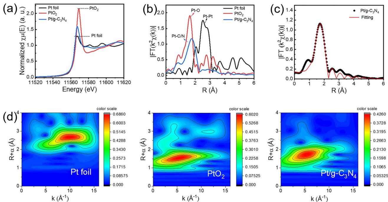
Fig. 3 XAFS results of Pt/g-C<sub>3</sub>N<sub>4</sub> compared with Pt foil and PtO<sub>2</sub>. (a) XANES spectra. (b) FT-EXAFS spectra. (c) FT-EXAFS fitting through Pt–N. (d) WT-EXAFS spectra.
