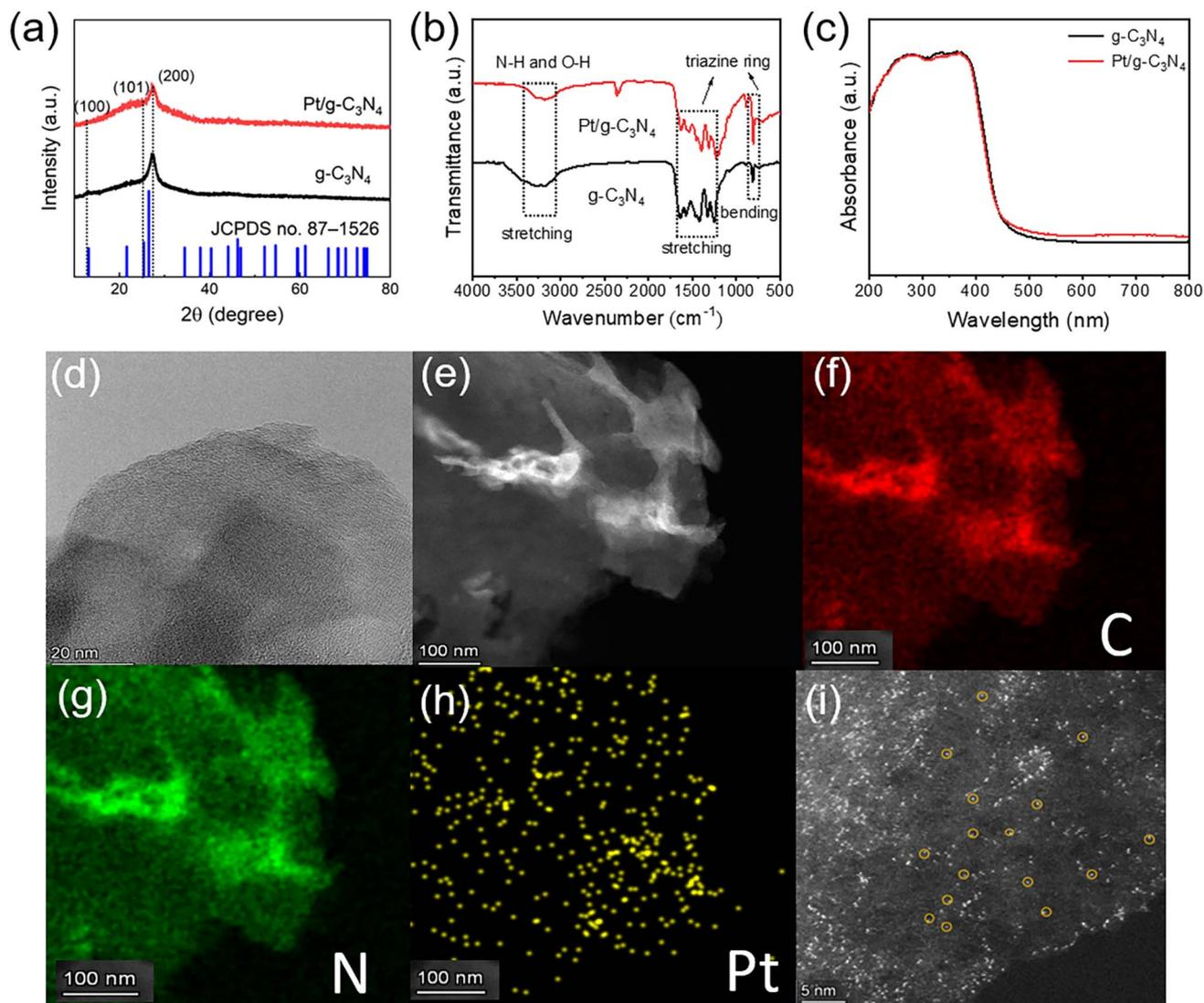
Fig. 1 Microstructures of few-layer  $g\text{-C}_3\text{N}_4$  and  $\text{Pt}/g\text{-C}_3\text{N}_4$ . (a) XRD patterns. (b) FTIR spectra. (c) DRS spectra. (d) High-resolution TEM image of  $\text{Pt}/g\text{-C}_3\text{N}_4$ . (e–h) Elemental mapping profiles of  $\text{Pt}/g\text{-C}_3\text{N}_4$  under the dark-field of HAADF-STEM (e), C (f), N (g), and Pt (h). (i) High-resolution HAADF-STEM image under dark-field to clearly demonstrate Pt single atoms.
