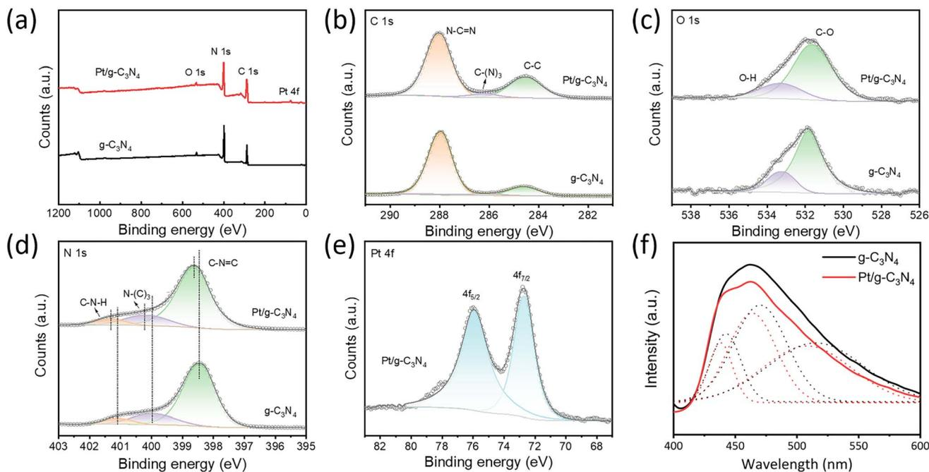
Fig. 2 Chemical state of few-layer  $g\text{-C}_3\text{N}_4$  and  $\text{Pt}/g\text{-C}_3\text{N}_4$ . (a–e) XPS spectra of survey (a), C 1s (b), O 1s (c), N 1s (d), and Pt 4f (e). (f) PL spectra.
