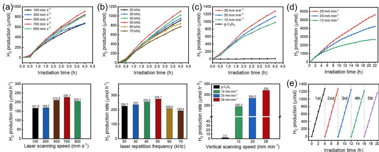
Fig. 4 The photocatalytic hydrogen evolution performance of Pt/g-C<sub>3</sub>N<sub>4</sub> under different synthetic conditions. (a) Effect of laser scanning speed. (b) Effect of laser repetition frequency. (c) Effect of vertical scanning speed. (d) Prolonged photocatalytic test over 22 h. (e) Photocatalytic capabilities within five cycles.
