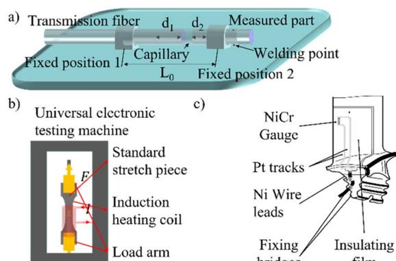
Fig. 8 Strain gauges for aerospace applications: (a) conceptual diagram illustrating the installation of a FBG strain gauge on a metallic shell;<sup>38</sup> (b) inductive heating-type universal testing machine incorporating standard tensile specimens; (c) schematic representation of the fabrication of a NiCr TFSG on a turbine blade.<sup>85</sup>
