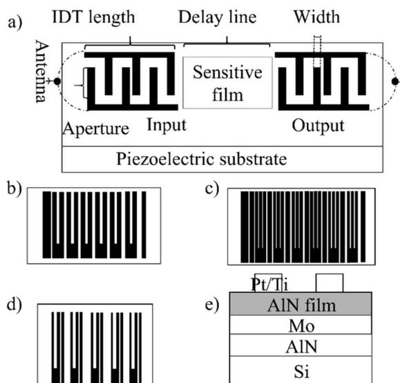
Fig. 2 Structure of SAW high-temperature strain gauges: (a) basic structure;<sup>23</sup> (b) structure diagram of a conventional interdigital electrode;<sup>26</sup> (c) structure diagram of a split interdigital electrode;<sup>26</sup> (d) single phase transducer;<sup>26</sup> (e) structure diagram of a Pt/Ti/AlN/Mo/AlN/Si sensor.<sup>30</sup>
