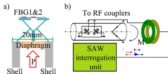
Fig. 7 Application of high-temperature strain gauge: (a) schematic diagram of the application of an optical fiber grating high-temperature strain gauge in oil wells;<sup>82</sup> (b) SAW high-temperature strain gauge in the application diagram in the automotive industry.<sup>85</sup>
