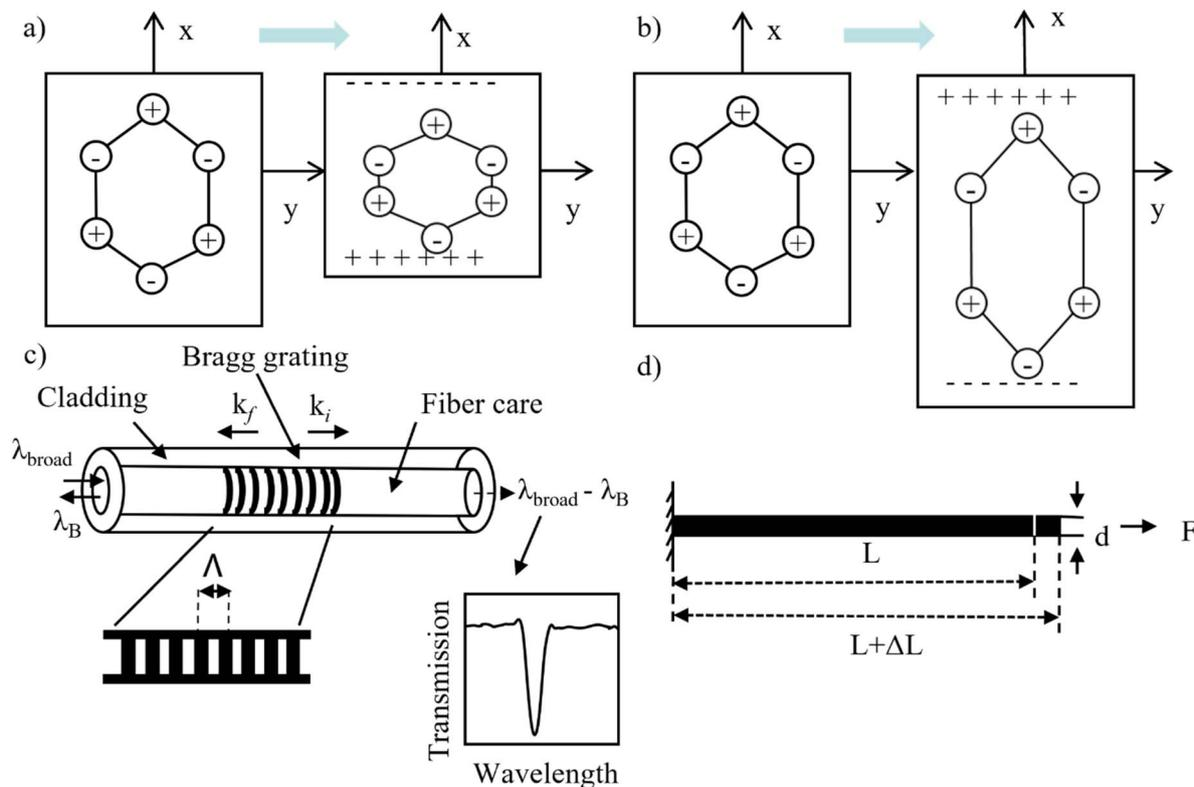
Fig. 1 Schematic diagram of a high-temperature strain gauge: (a) positive piezoelectric effect;<sup>15</sup> (b) negative piezoelectric effect;<sup>15</sup> (c) uniform optical fiber grating structure; (d) schematic diagram of the strain effect of a high-temperature TFSG.
