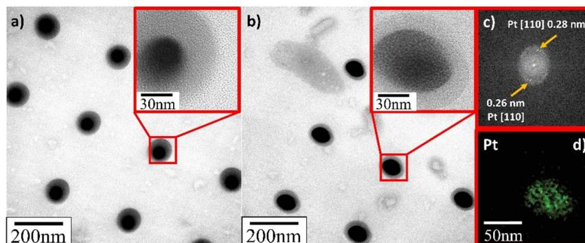
Fig. 8 TEM and HR-TEM images of deposited Pt NPs on TOGO sheets for deposition time: (a) 0.3 s; (b) 1.0 s; (c) FFT pattern calculated from HR-TEM image in Fig. S3;† (d) EDS elemental map of platinum.
