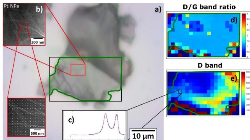
Fig. 12 Raman characterization of deposited Pt NPs on HUGO sheet: (a) optical image of HUGO sheet with highlighted area of interest by green outline; (b) SEM image of deposited Pt NP precise spot studied via Raman mapping due to correlative approach; (c) Raman spectrum. Raman 2D contour plot of same spot from optical image highlighted by black rectangle: (d) D/G band ratio; (e) D band.
