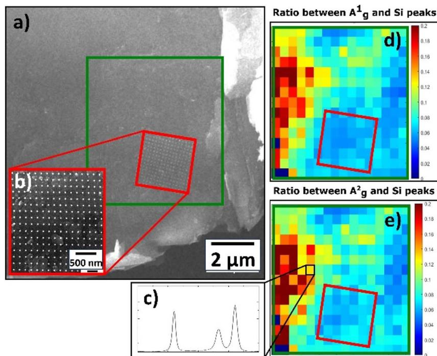
Fig. 13 Raman characterization of deposited Pt NPs on BP: (a) SEM image of BP sheet with highlighted area of interest by green rectangle; (b) SEM image of Pt NP precise spot studied *via* Raman mapping due to correlative approach; (c) Raman spectrum. Raman 2D contour plot of same spot from SEM image highlighted by green rectangle: (d)  $A_{1g}^1$  band ratio; (e)  $A_{2g}^2$  band ratio.
