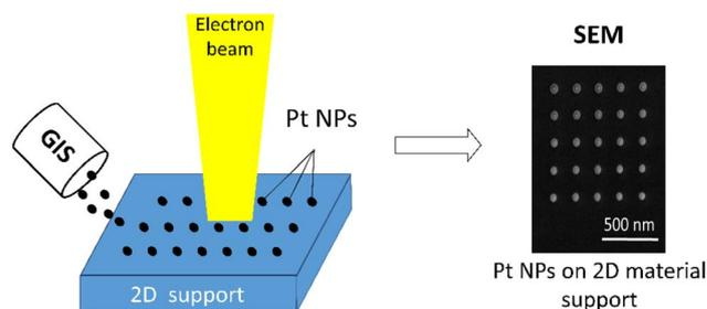
Fig. 1 Illustration of Pt deposition onto 2D support by EBL.
