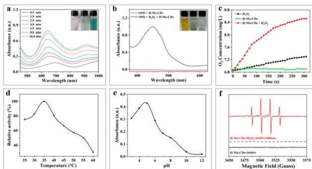
Fig. 3 Time-dependent absorbance changes of TMB after different treatments (a); the UV-Vis absorbance changes of OPD (b); time-dependent  $O_2$  production of  $H_2O_2$ , H-Mo-CDs, and H-Mo-CDs +  $H_2O_2$  in water (c); effect of temperature on peroxidase activity of H-Mo-CDs (d); pH-dependent absorbance changes of H-Mo-CDs +  $H_2O_2$  (e); ESR spectra of DMPO after different treatments (f).
