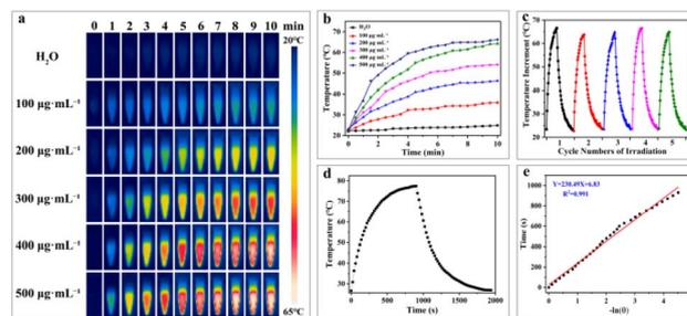
Fig. 2 The corresponding time-dependent photothermal curves of samples (a) and photothermal images of H-Mo-CDs and water upon exposure to an 808 nm laser for different time periods (b); heating/cooling curve of H-Mo-CDs over five cycles (c); a single heating/cooling curve (d) and the corresponding plot of cooling time vs. the negative natural logarithm of driving force temperature (e). ( $808 \text{ nm}$ ,  $0.8 \text{ W cm}^{-2}$ ).
