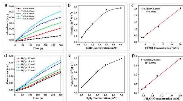
Fig. 4 Steady-state kinetic assay of H-Mo-CDs. Time-dependent absorbance changes at 652 nm of TMB reaction solutions catalyzed by H-Mo-CDs in the presence of different concentrations of TMB (a) or  $H_2O_2$  (d). The velocity ( $v$ ) of the reaction changes in the presence of different concentrations of TMB (b) or  $H_2O_2$  (e). Double reciprocal plots of the activity of H-Mo-CDs in the presence of different concentrations of TMB (c) or  $H_2O_2$  (f).
