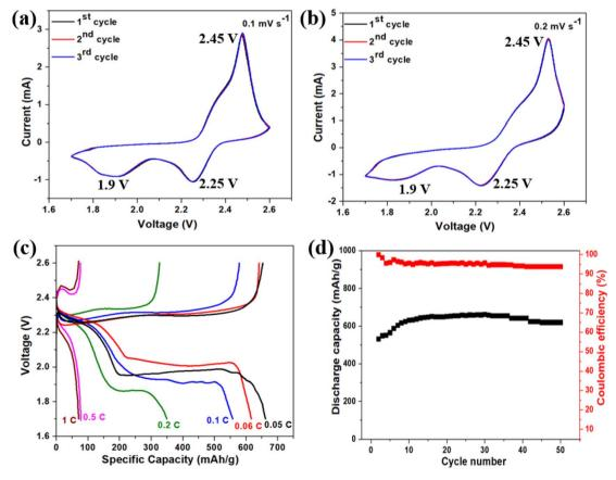
Fig. 8 The electrochemical characterization of sulfur-BAC composite-based cathode. The cyclic voltammetry profile of sulfur-BAC composite-based cathode at a scan rate of (a)  $0.1\,\text{mV}\,\text{s}^{-1}$  and (b)  $0.2\,\text{mV}\,\text{s}^{-1}$ . (c) The charge-discharge sulfur-BAC composite-based cathodes at various C-rates (0.05-1C). (d) The cyclic stability and coulombic efficiency of sulfur-BAC composite-based cathode over 50 cycles.
