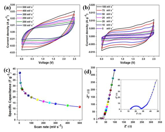
Fig. 5 The electrochemical characterization of BAC-based SCSD. (a and b) The cyclic voltammetry profile of BAC-based SCSD was measured at various scan rates (5–500 mV s<sup>-1</sup>). (c) Effect of the gravimetric specific capacitance of BAC-based SCSD with respect to scan rates. (d) The Nyquist plot of BAC-based SCSD and the inset shows the enlarged view of the Nyquist plot.
