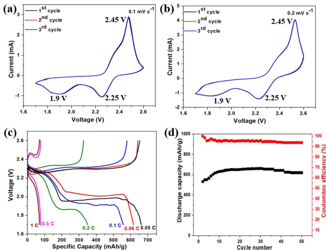
Fig. 8 The electrochemical characterization of sulfur-BAC composite-based cathode. The cyclic voltammetry profile of sulfur-BAC composite-based cathode at a scan rate of (a)  $0.1 \text{ mV s}^{-1}$  and (b)  $0.2 \text{ mV s}^{-1}$ . (c) The charge-discharge sulfur-BAC composite-based cathodes at various C-rates (0.05–1C). (d) The cyclic stability and coulombic efficiency of sulfur-BAC composite-based cathode over 50 cycles.
