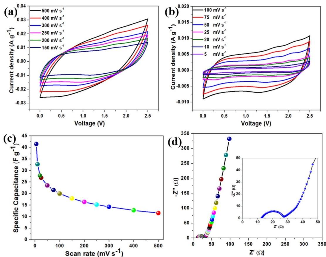
Fig. 5 The electrochemical characterization of BAC-based SCSD. (a and b) The cyclic voltammetry profile of BAC-based SCSD was measured at various scan rates (5–500 mV s<sup>-1</sup>). (c) Effect of the gravimetric specific capacitance of BAC-based SCSD with respect to scan rates. (d) The Nyquist plot of BAC-based SCSD and the inset shows the enlarged view of the Nyquist plot.
