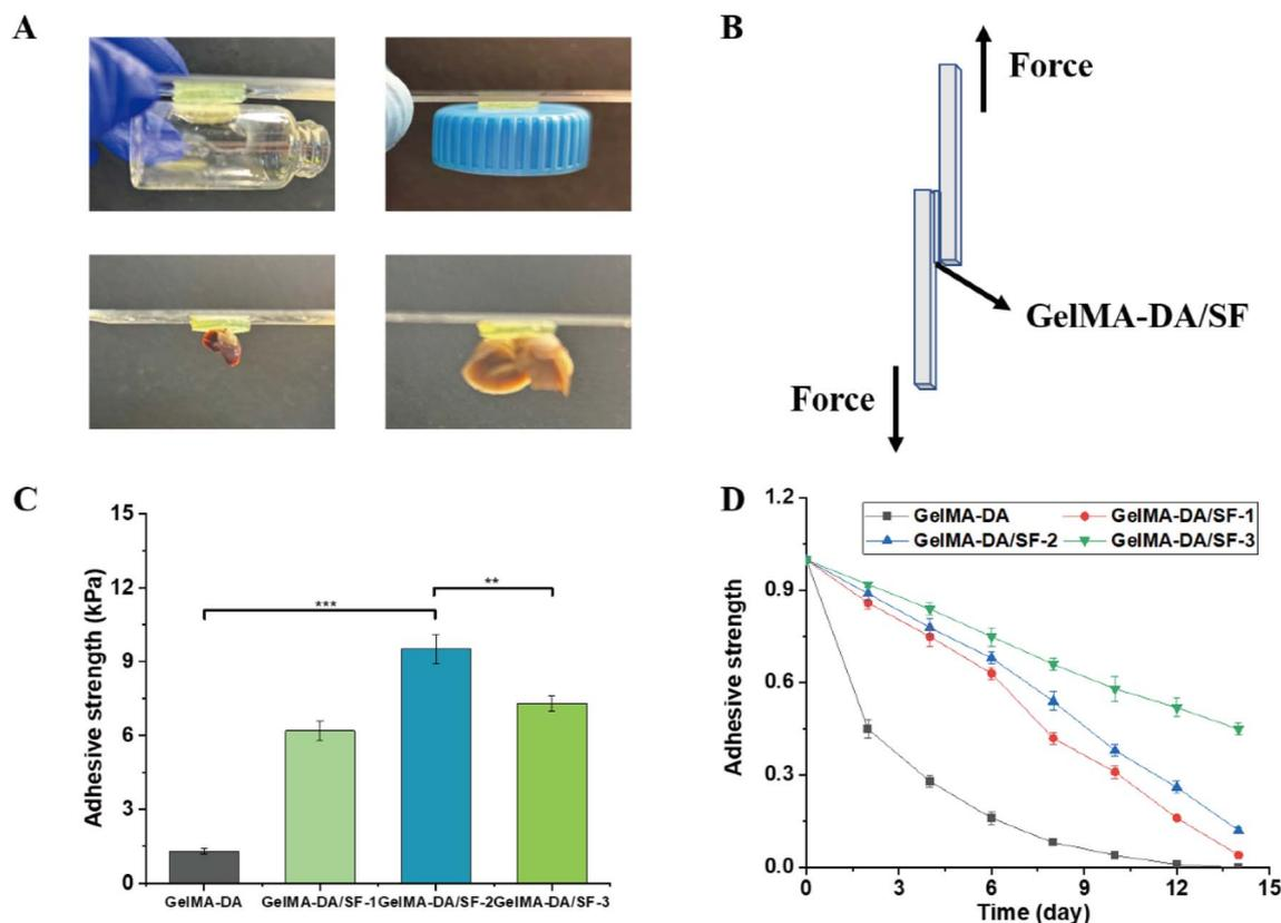
Fig. 4 Adhesion properties of the GelMA-DA/SF hydrogel. (A) GelMA-DA/SF hydrogel can adhere to various material surfaces (glass, plastic, etc.) and can also attach rat organs to glass. (B) Schematic diagram of the adhesion strength testing of the GelMA-DA/SF hydrogel. (C) Adhesion strength of the GelMA-DA/SF hydrogel with different compositions. (D) Adhesion strength of materials with different compositions over time. ( $n \geq 3$ ), \*\*,  $p < 0.01$ , \*\*\* $p < 0.001$ .
