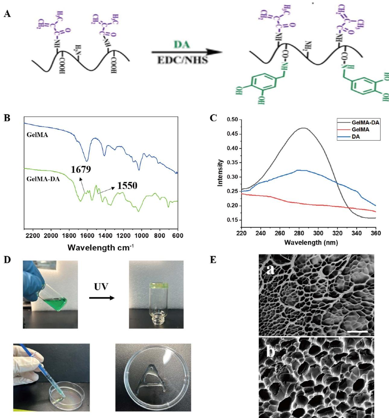
Fig. 2 Characterization of the GelMA-DA/SF hydrogel. (A) Schematic of GelMA-DA synthesis. (B) Infrared spectra of GelMA and GelMA-DA. (C) UV spectra of GelMA and GelMA-DA. (D) Demonstration of the GelMA-DA/SF hydrogel's rapid photopolymerization and injectability. (E) Typical scanning electron microscopy (SEM) image of (a) GelMA-DA/SF and (b) GelMA-DA hydrogels. Scale bar, 100  $\mu\text{m}$ .
