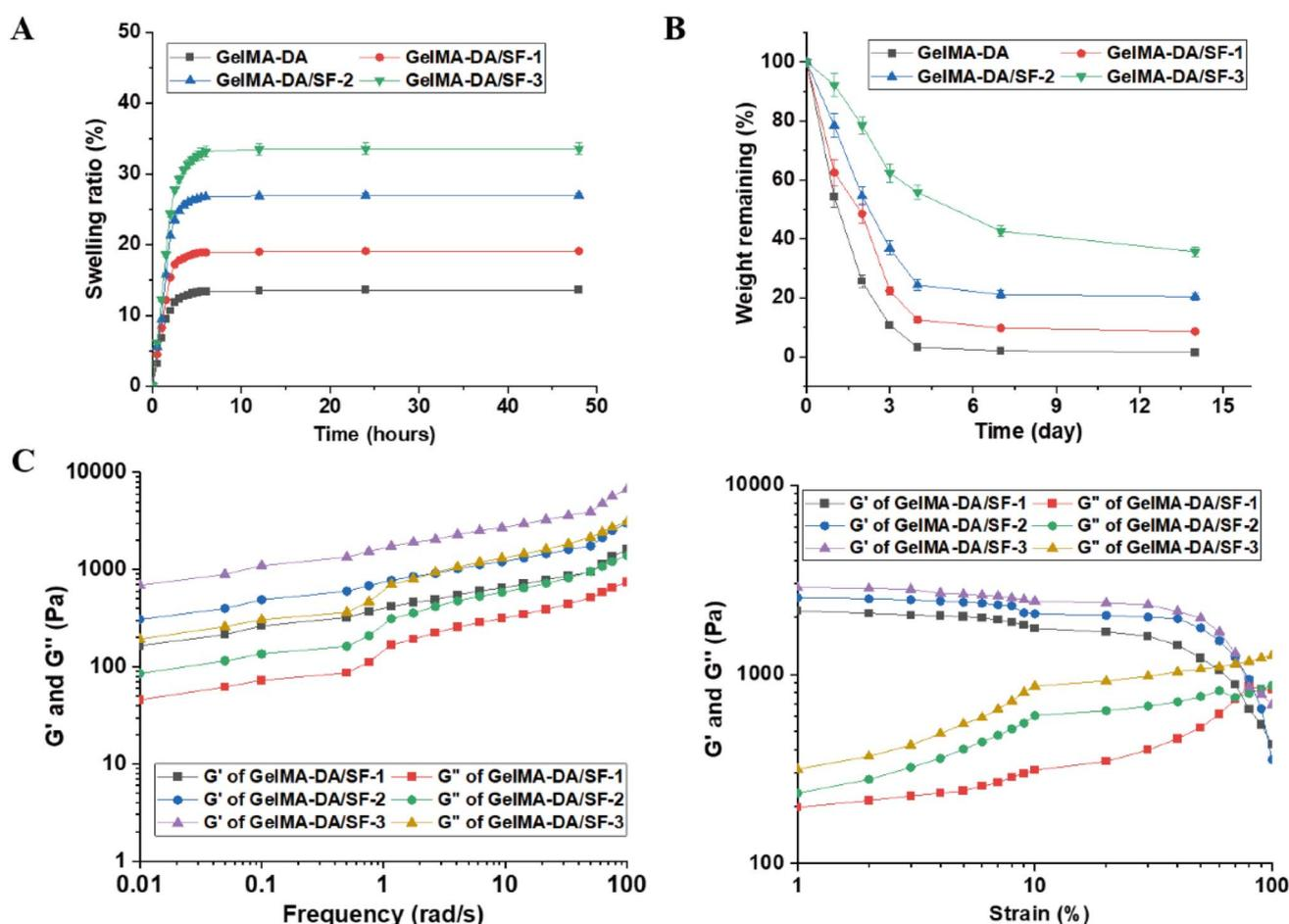
Fig. 3 Mechanical properties of the GelMA-DA/SF hydrogel. (A) Swelling curves and (B) degradation curves of hydrogels with different compositions. (C) Rheological properties of hydrogels with different compositions under two modes.
