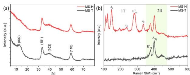
Fig. 1 (a) XRD patterns and (b) Raman spectra of 2H MoS<sub>2</sub> (MS-H) and 1T MoS<sub>2</sub> (MS-T).
