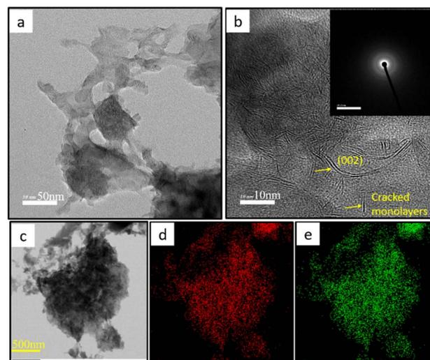
Fig. 4 (a) TEM image of the MS-T sample, (b) HR-TEM image of lattice fringe spacing and the SAED pattern (inset in (b)), and (c–e) STEM elemental mapping of the MoS<sub>2</sub> sample: (c) greyscale image, (d) Mo-K $\alpha$ , and (e) S-K $\alpha$  of MS-T.
