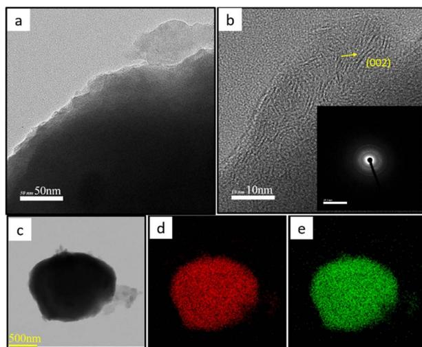
Fig. 3 (a) TEM image of the MS-H sample, (b) HR-TEM image of lattice fringe spacing and the SAED pattern (inset in (b)), and (c–e) STEM elemental mapping of the MoS<sub>2</sub> sample: (c) greyscale image, (d) Mo-K $\alpha$ , and (e) S-K $\alpha$  of MS-T.
