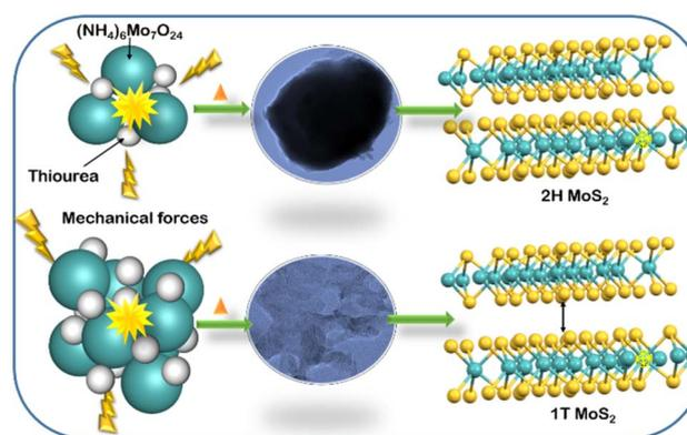
Fig. 5 Schematic illustration of the formation of 2H and 1T MoS<sub>2</sub>.
