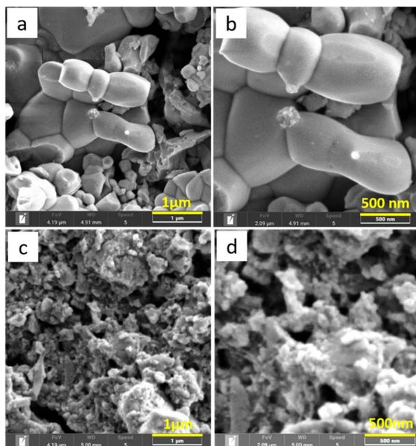
Fig. 2 FESEM images of MoS<sub>2</sub> samples: (a and b) MS-H and (c and d) MS-T.
