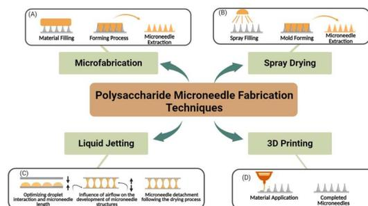
Fig. 4 Microneedle preparation technologies. (A) Microfabrication (B) spray drying (C) liquid jetting (D) 3D printing.
