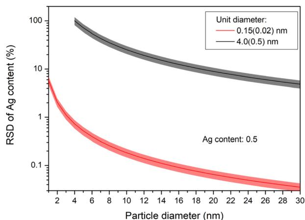
Fig. 1 The variation of RSD as a function of (final) particle diameter at two different unit diameters. The shadowed areas around the lines represent the uncertainty due to the uncertainty in the unit particle diameter. Please note the logarithmic scale in the vertical axis.
