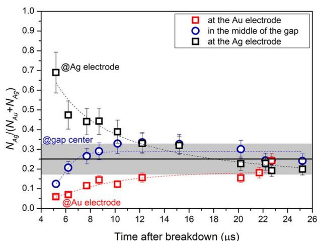
Fig. 6 Variation of the plasma composition – defined as the Ag content in atomic ratio – in time at different positions along the spark gap. The black line indicates the average composition of the AuAg BNPs forming under the same conditions, with a grey zone representing the  $\text{SD}_\phi$  of the obtained composition distribution. The positional accuracy of the light collecting slit is estimated to be not worse than 85  $\mu\text{m}$ .
