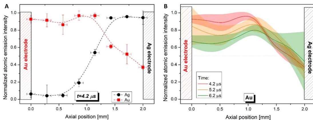
Fig. 4 Spatial distribution of atomic emission intensity of Au and Ag atoms along the spark gap 4.2  $\mu\text{s}$  after the onset of the breakdown (A). Temporal variation of the spatial intensity distribution of Au atomic emission intensity (B). Measured points are connected to guide the eye.
