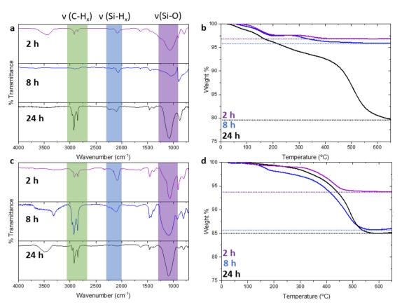
Fig. 3 (a) FT-IR spectra of dodecyl-terminated Si NPs obtained from sonochemical reactions in the absence of a radical initiator for 2 h (purple), 8 h (blue), and 24 h (black) with (b) corresponding TGA data. (c) FT-IR spectra of dodecyl-terminated Si NPs recovered from reactions involving AIBN for 2 h (purple), 8 h (blue), and 24 h (black) with (d) corresponding TGA data.
