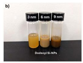
Fig. 5 Qualitative appearance of toluene suspensions containing unfunctionalized Si-H and functionalized dodecyl Si-NPs of indicated sizes for reactions after 2 h of sonication (a) with and (b) without AIBN radical initiator.
