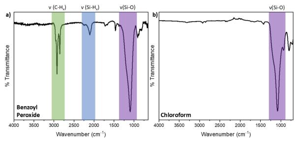
FT-IR Spectra of 9 nm dodecyl-functionalized SiNPs sonicated for 24 h with (a) benzoyl peroxide and (b) chloroform.
