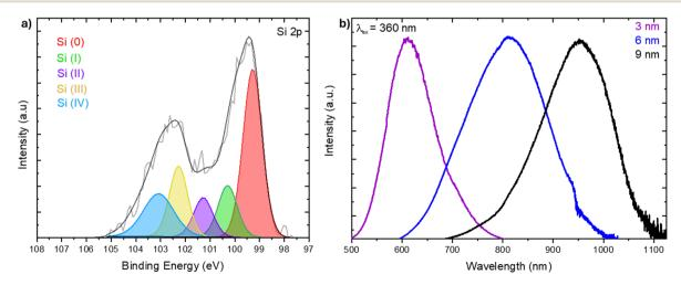
Fig. 2 (a) High resolution Si 2p XP spectrum of 9 nm dodecyl SiNPs sonicated for 24 h. Si 2p<sub>1/2</sub> envelopes omitted for clarity. (b) Normalized photoluminescence spectra of 3 (purple), 6 (blue), and 9 (black) nm dodecyl-SiNPs sonicated for 24 h.
