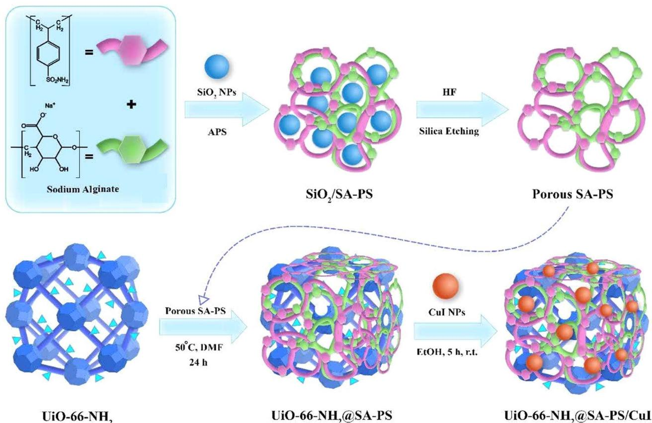
Scheme 2 Schematic pathway for the fabrication of UiO-66-NH<sub>2</sub>@SA-PS/CuI.<sup>31</sup>
