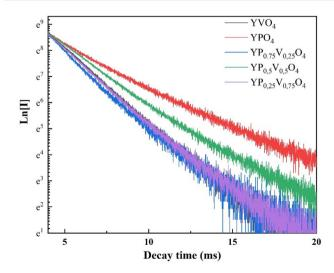
Fig. 8 Luminescence decay curves for Y(P<sub>1-x</sub>V<sub>x</sub>)O<sub>4</sub>:5% Eu.
