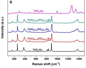
Fig. 2 (A) FTIR and (B) Raman spectra of  $YP_{(1-x)}V_xO_4:5\%$  Eu materials.
