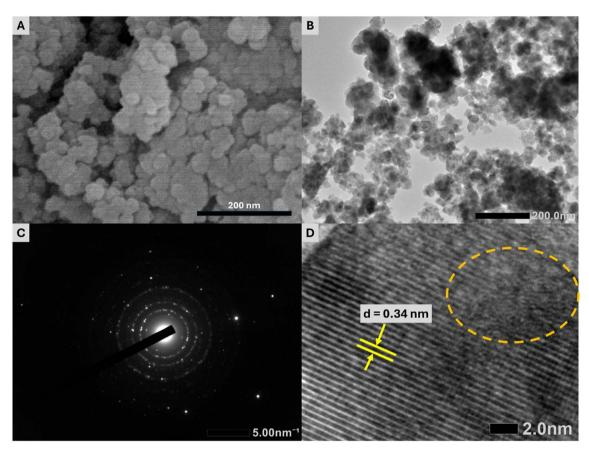
Fig. 3 (A) SEM, (B) TEM, (C) SAED, and (D) HR-TEM images of the  $Y(P_{0.5}V_{0.5})O_4$ :5% Eu sample.
