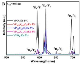
Fig. 7 Fluorescence spectra of  $Y(P_{1-x}V_x)O_4$ :5% Eu samples under (A) 320 nm and (B) 395 nm excitation.
