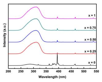
Fig. 5 Fluorescence excitation spectrum of  $Y(P_{1-x}V_x)O_4$ :5% Eu materials (x = 0, 0.25, 0.5, 0.75,and 1).
