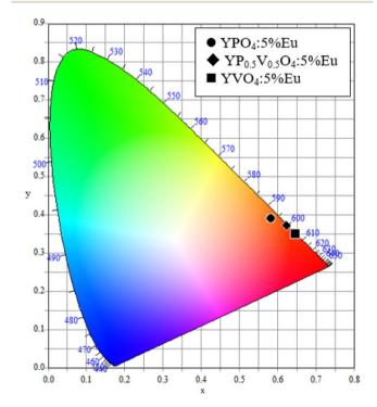
Fig. 9 CIE chromaticity diagram for emission spectra of  $YP_{(1-x)}V_{x}-Q_{4}$ :5% Eu<sup>3+</sup> (x=0,0.5,1).
