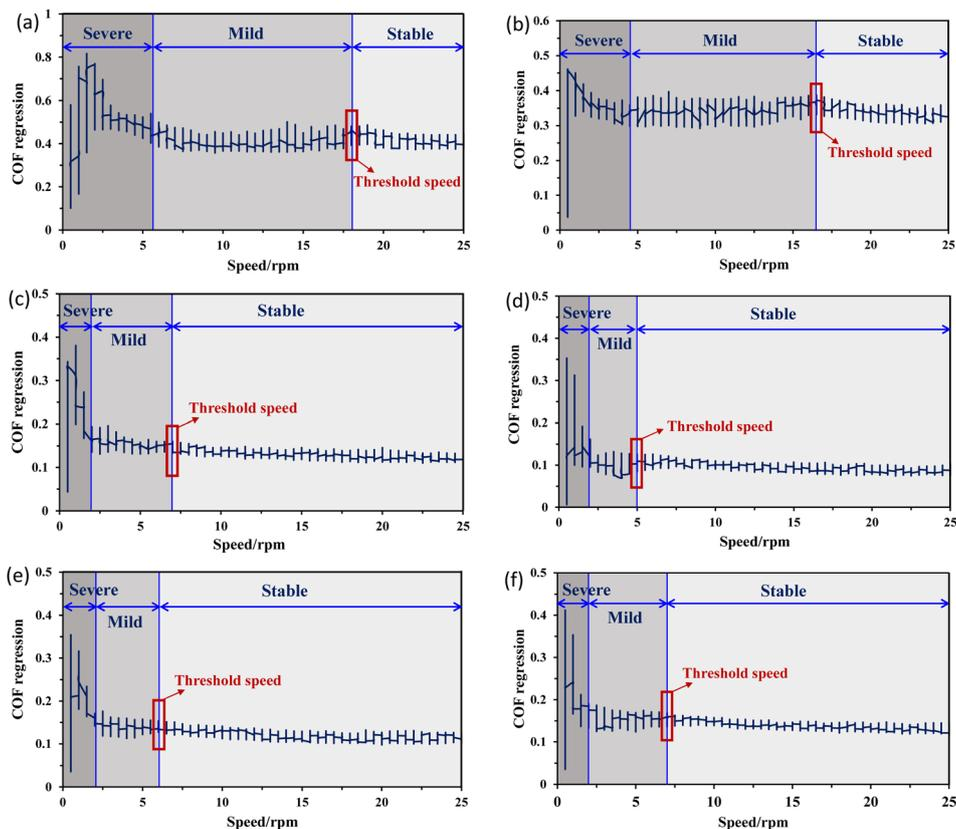
Fig. 8 COF regression vs. speed under 50 N force for 50 min using different conditions: (a) dry, (b) water, (c) 0.25 wt% hBN/TiO<sub>2</sub>, (d) 0.5 wt% hBN/TiO<sub>2</sub>, (e) 1.0 wt% hBN/TiO<sub>2</sub>, and (f) 2.0 wt% hBN/TiO<sub>2</sub>.
