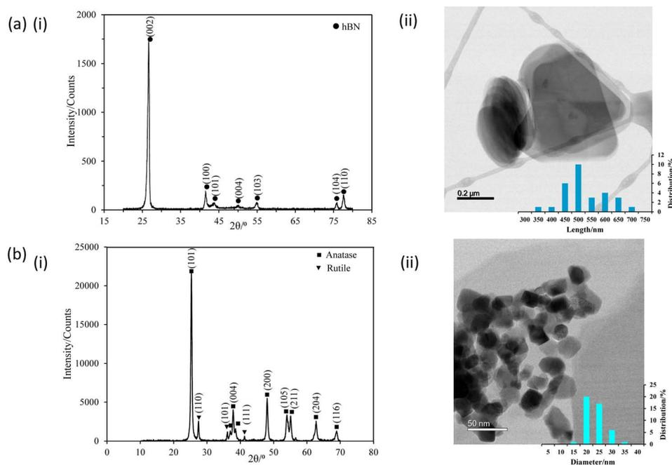
Fig. 3 (i) XRD patterns and (ii) TEM images with size distributions of (a) hBNNSs and (b) P25 TiO<sub>2</sub> NPs.
