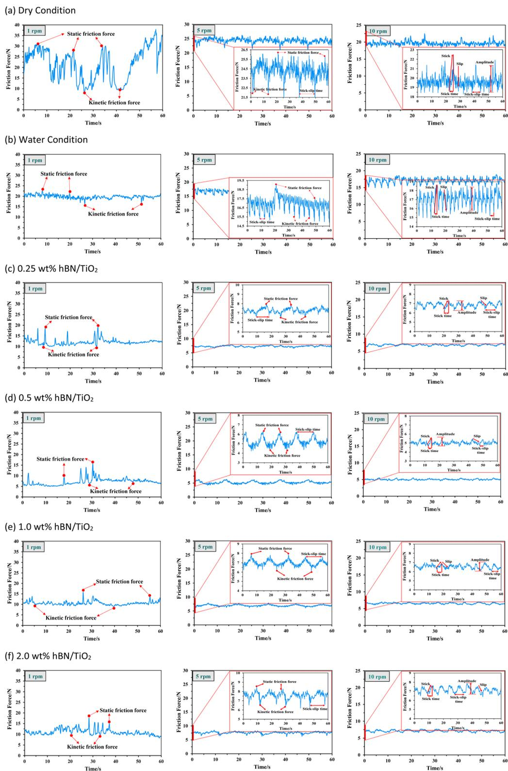
Fig. 6 The variation of friction forces over time at 1, 5, and 10 rpm under 50 N force for different conditions, (a) dry, (b) water, (c) 0.25 wt% hBN/TiO<sub>2</sub>, (d) 0.5 wt% hBN/TiO<sub>2</sub>, (e) 1.0 wt% hBN/TiO<sub>2</sub>, and (f) 2.0 wt% hBN/TiO<sub>2</sub>.
