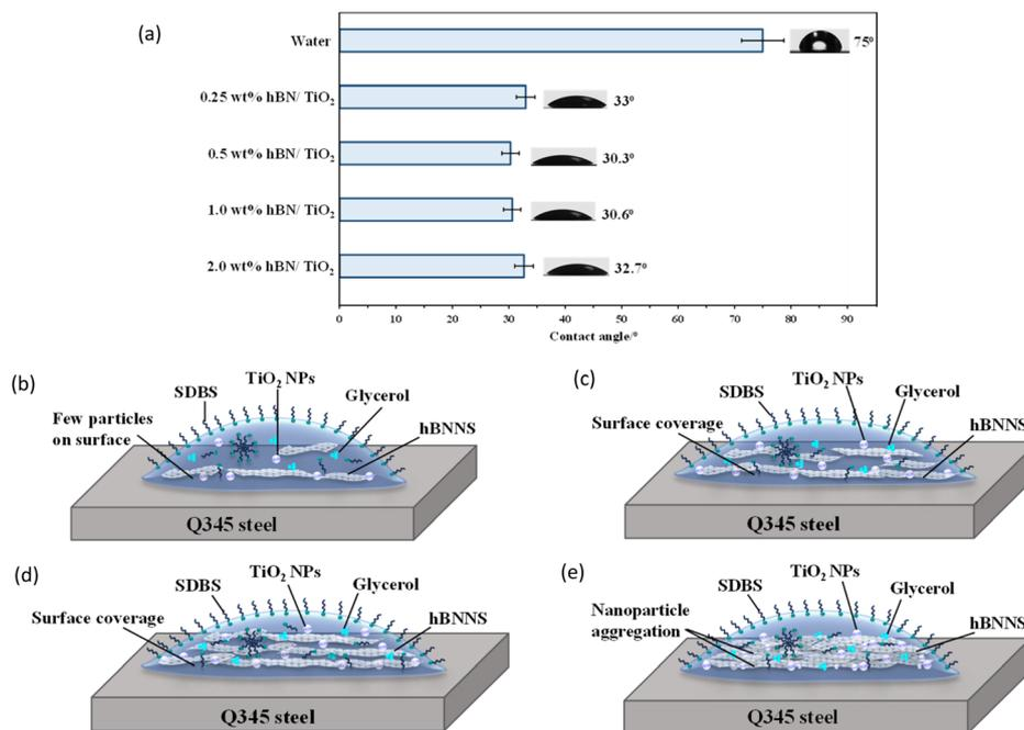
Fig. 11 (a) Contact angle measured on the Q345 steel surface using various lubricants; the schematic diagram of contact angles when lubricated with (b) 0.25 wt% hBN/TiO<sub>2</sub>, (c) 0.5 wt% hBN/TiO<sub>2</sub>, (d) 1.0 wt% hBN/TiO<sub>2</sub>, and (e) 2.0 wt% hBN/TiO<sub>2</sub>.
