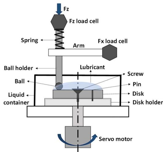
Fig. 2 Schematic illustration of the ball-on-disk tribometer setup.<sup>27</sup>
