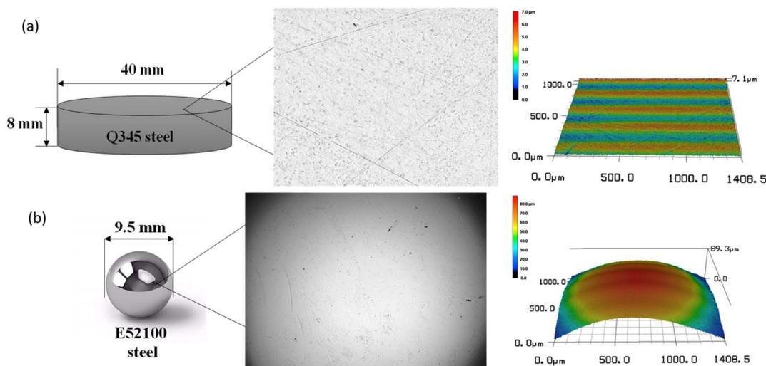
Fig. 1 Schematic, optical image, and 3D profile of the (a) disk and (b) ball.<sup>27</sup>
