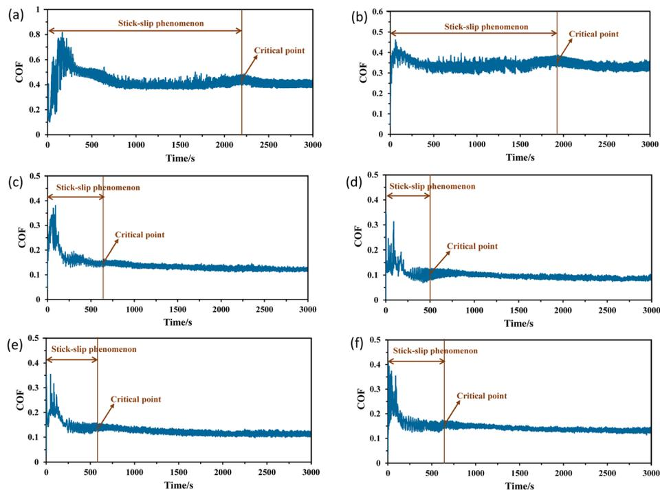
Fig. 4 COF vs. time measured during tribological tests under different lubricating conditions, (a) dry, (b) water, (c) 0.25 wt% hBN/TiO<sub>2</sub>, (d) 0.5 wt% hBN/TiO<sub>2</sub>, (e) 1.0 wt% hBN/TiO<sub>2</sub>, and (f) 2.0 wt% hBN/TiO<sub>2</sub>, revealing the stick–slip phenomenon (50 N, 0–25 rpm).
