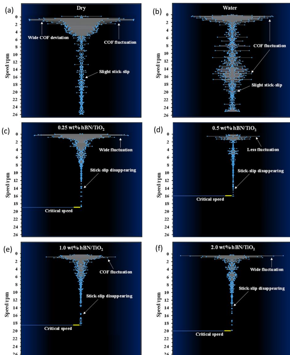
Fig. 10 COF deviation vs. speed under 50 N for 50 min when lubricated with (a) dry, (b) water, (c) 0.25 wt% hBN/TiO<sub>2</sub>, (d) 0.5 wt% hBN/TiO<sub>2</sub>, (e) 1.0 wt% hBN/TiO<sub>2</sub>, and (f) 2.0 wt% hBN/TiO<sub>2</sub>.
