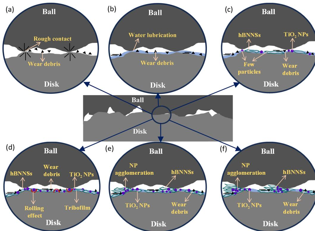
Fig. 15 Schematics of lubrication mechanisms during ball-on-disk tribological testing under (a) dry, (b) water, (c) 0.25 wt% hBN/TiO<sub>2</sub>, (d) 0.5 wt% hBN/TiO<sub>2</sub>, (e) 1.0 wt% hBN/TiO<sub>2</sub>, and (f) 2.0 wt% hBN/TiO<sub>2</sub>.
