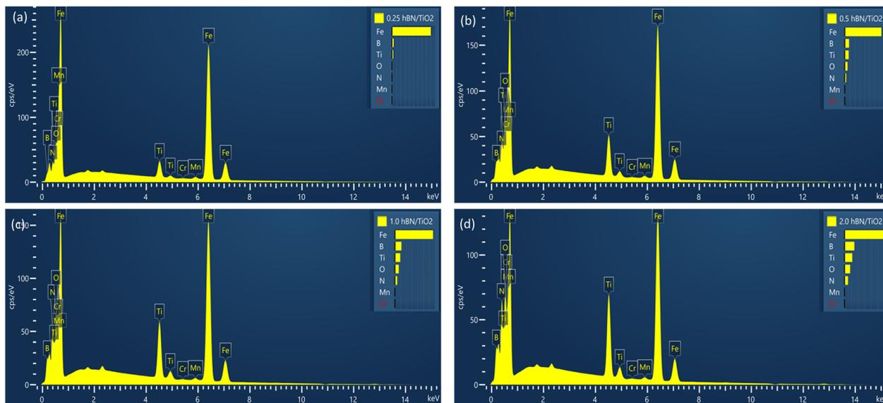
Fig. 14 EDS spectra of disk wear when lubricated with (a) 0.25 wt% hBN/TiO<sub>2</sub>, (b) 0.5 wt% hBN/TiO<sub>2</sub>, (c) 1.0 wt% hBN/TiO<sub>2</sub>, and (d) 2.0 wt% hBN/TiO<sub>2</sub> (50 N, 0–25 rpm, 50 min).
