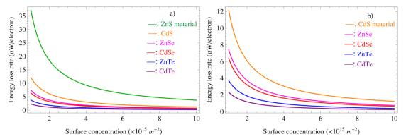
Fig. 6 Comparison of the surface concentration dependence of the electron ELR between Zn X and Cd X materials (X = Te, X, and X) when interacting with optical phonons. Here, the lattice temperature,  $T_{\ell}=4.2$  K, the electronic effective temperature,  $T_{E}=77$  K, the quantizing magnetic field,  $B_{Q}$ , is taken at the value which satisfies the MPR condition with n = 1, as shown in the discussion of Fig. 1, and the material slab thickness,  $D_z = 7$  nm.
