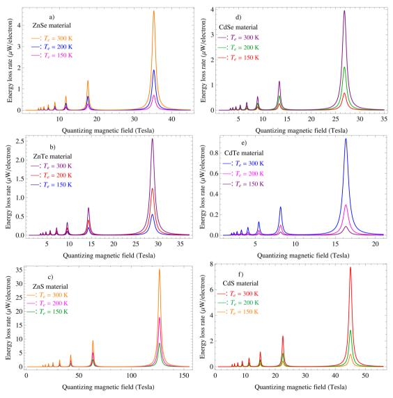
Fig. 2 Comparison of the quantizing magnetic field dependence of the electron ELR between Zn X and Cd X materials (X = Te, S, and Se) when interacting with optical phonons at various effective temperatures,  $T_{E} = 150$  K,  $T_{E} = 200$  K, and  $T_{E} = 300$  K. Here, the lattice temperature,  $T_{\ell} = 4.2$ K, the surface concentration,  $N_s = 2 \times 10^{15} \text{ m}^{-2}$ , and the material slab thickness,  $D_z = 7 \text{ nm}$ .
