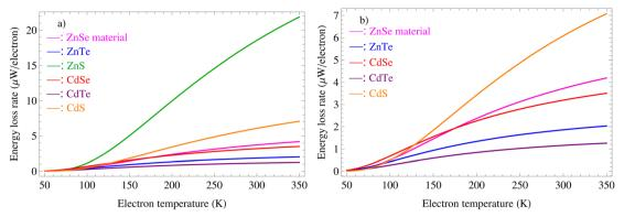
Fig. 3 Comparison of the electronic effective temperature dependence of the electron ELR between Zn X and Cd X materials (X = Te, S, and Se) when interacting with optical phonons. Here, the lattice temperature,  $T_\ell = 4.2$  K, the material slab thickness,  $D_Z = 10$  nm, the surface concentration,  $N_S = 2 \times 10^{15}$  m $^{-2}$ , and the quantizing magnetic field,  $B_Q$ , is taken at the value which satisfies the MPR condition with n = 1, as shown in the discussion of Fig. 1.
