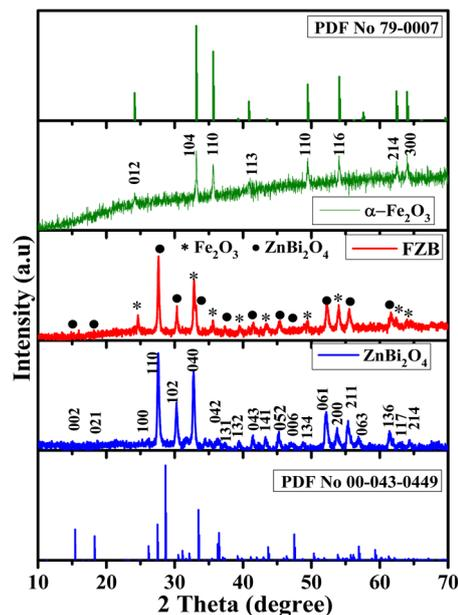
Fig. 1 XRD patterns of  $\alpha$ -Fe<sub>2</sub>O<sub>3</sub>, ZBO, and FZB.
