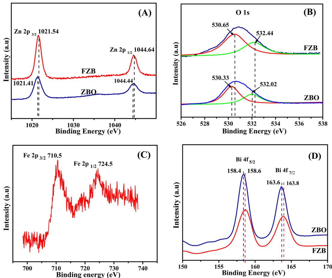
Fig. 4 XPS spectra of (A) FZB heterojunction and high-resolution (B) O 1s, (C) Fe 2p, and (D) Bi 4f XPS spectra.
