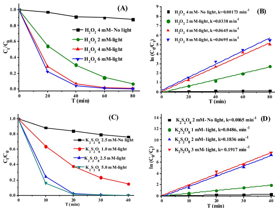
Fig. 7 Effect of  $\text{H}_2\text{O}_2$  (A) and (B) and  $\text{K}_2\text{S}_2\text{O}_8$  (C) and (D) on MB degradation using the FZB heterojunction under visible light.
