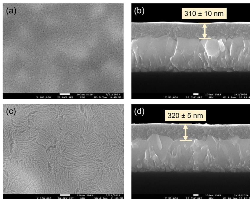
Fig. 2 Surface FESEM of (a) compact and (c) mesoporous  $\text{TiO}_2$  films, and cross-sectional images of (b) compact and (d) mesoporous  $\text{TiO}_2$  films.
