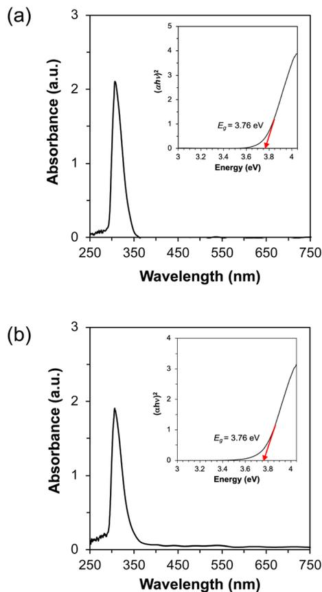
Fig. 5 Optical absorption spectra of (a) compact and (b) mesoporous TiO<sub>2</sub> films. The insets show estimated band gaps from the optical absorption spectra of both films.
