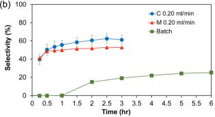
Fig. 10 (a) Highest conversion of benzyl alcohol and (b) highest selectivity of benzaldehyde using the compact TiO<sub>2</sub> film and mesoporous TiO<sub>2</sub> film as photoanodes obtained from the PEC flow cell compared with that of the batch setup
