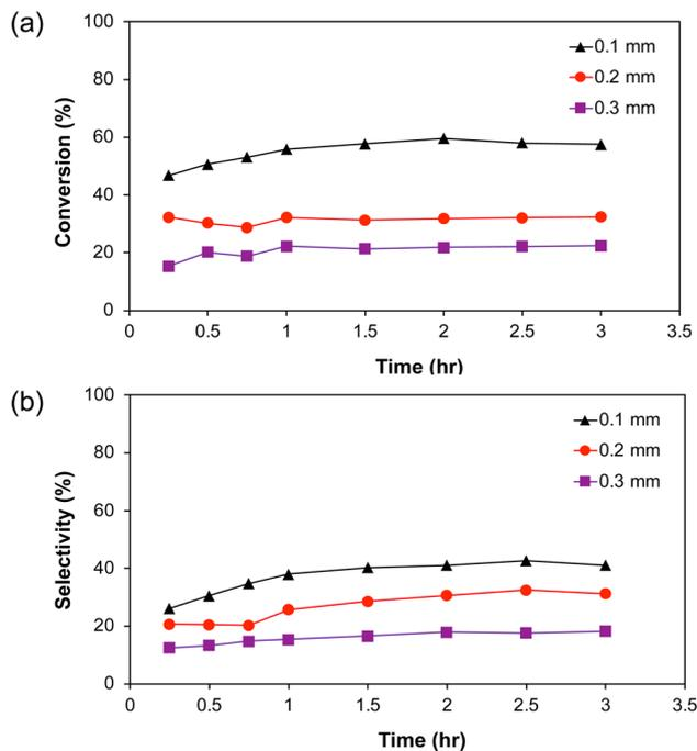
Fig. 8 (a) Conversion of benzyl alcohol and (b) selectivity of benzaldehyde obtained at a fixed flow rate of 0.10 ml min<sup>-1</sup> using the compact TiO<sub>2</sub> film as the photoanode in the PEC flow cell with different channel widths.
