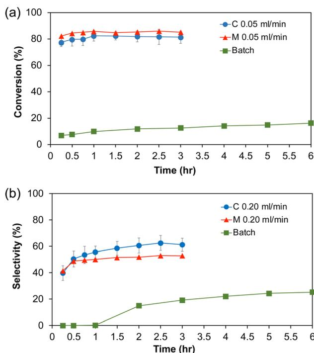
Fig. 10 (a) Highest conversion of benzyl alcohol and (b) highest selectivity of benzaldehyde using the compact TiO<sub>2</sub> film and mesoporous TiO<sub>2</sub> film as photoanodes obtained from the PEC flow cell compared with that of the batch setup.
