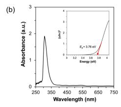
Fig. 5 Optical absorption spectra of (a) compact and (b) mesoporous  $TiO_2$  films. The insets show estimated band gaps from the optical absorption spectra of both films.
