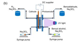
Fig. 1 Schematic diagram of the (a) components of the microchannel PEC flow cell and (b) experimental setup.
