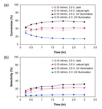
Fig. 6 (a) Conversion of benzyl alcohol and (b) selectivity of benzaldehyde obtained in the dark, in the presence of natural light and under UV illumination, and without applied voltage conditions, at a flow rate of 0.10 ml min<sup>-1</sup> using the compact TiO<sub>2</sub> film as the photoanode.
