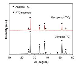
Fig. 3 XRD patterns of compact and mesoporous TiO<sub>2</sub> films deposited
