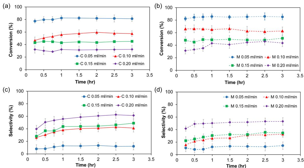
Fig. 9 Conversion of benzyl alcohol obtained from the reaction using (a) compact TiO<sub>2</sub> film and (b) mesoporous TiO<sub>2</sub> film, and selectivity of benzaldehyde obtained from the reaction using (c) compact TiO<sub>2</sub> film and (d) mesoporous TiO<sub>2</sub> film as photoanodes with various electrolyte flow rates.
