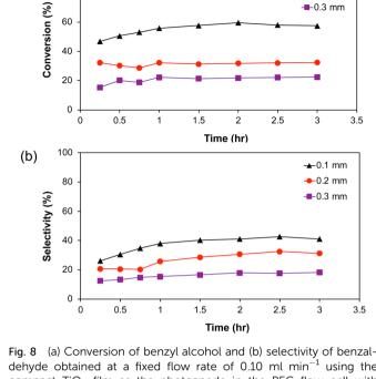
dehyde obtained at a fixed flow rate of 0.10 ml min<sup>-1</sup> using the compact TiO2 film as the photoanode in the PEC flow cell with different channel widths.
