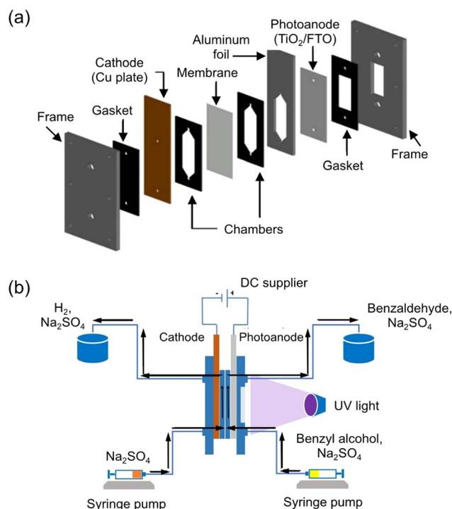
Fig. 1 Schematic diagram of the (a) components of the microchannel PEC flow cell and (b) experimental setup.
