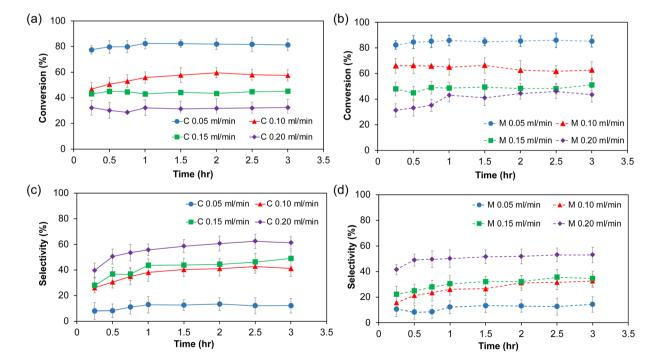
Conversion of benzyl alcohol obtained from the reaction using (a) compact TiO<sub>2</sub> film and (b) mesoporous TiO<sub>2</sub> film, and selectivity of benzaldehyde obtained from the reaction using (c) compact TiO<sub>2</sub> film and (d) mesoporous TiO<sub>2</sub> film as photoanodes with various electrolyte flow rates
