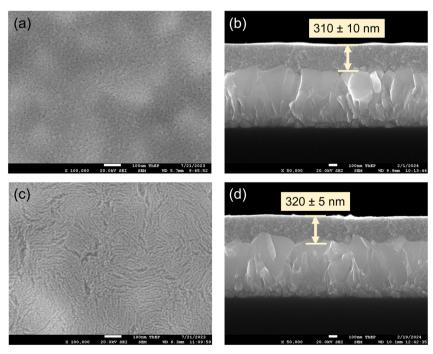
Fig. 2 Surface FESEM of (a) compact and (c) mesoporous TiO<sub>2</sub> films, and cross-sectional images of (b) compact and (d) mesoporous TiO<sub>2</sub> films.
