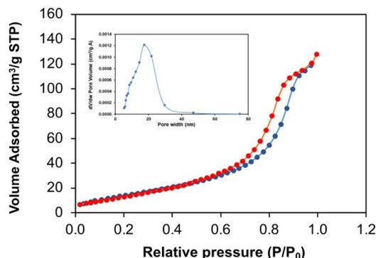
Fig. 4 Nitrogen adsorption/desorption isotherm of the mesoporous TiO<sub>2</sub> film. The inset shows the pore size distribution of the mesoporous TiO<sub>2</sub> film.
