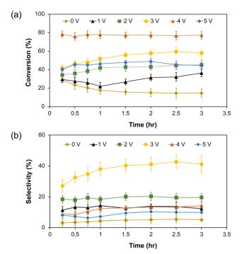
Fig. 7 (a) Conversion of benzyl alcohol and (b) selectivity of benzaldehyde obtained at a flow rate of 0.10 ml min<sup>-1</sup> using the compact TiO<sub>2</sub> film as the photoanode at different applied potentials.
