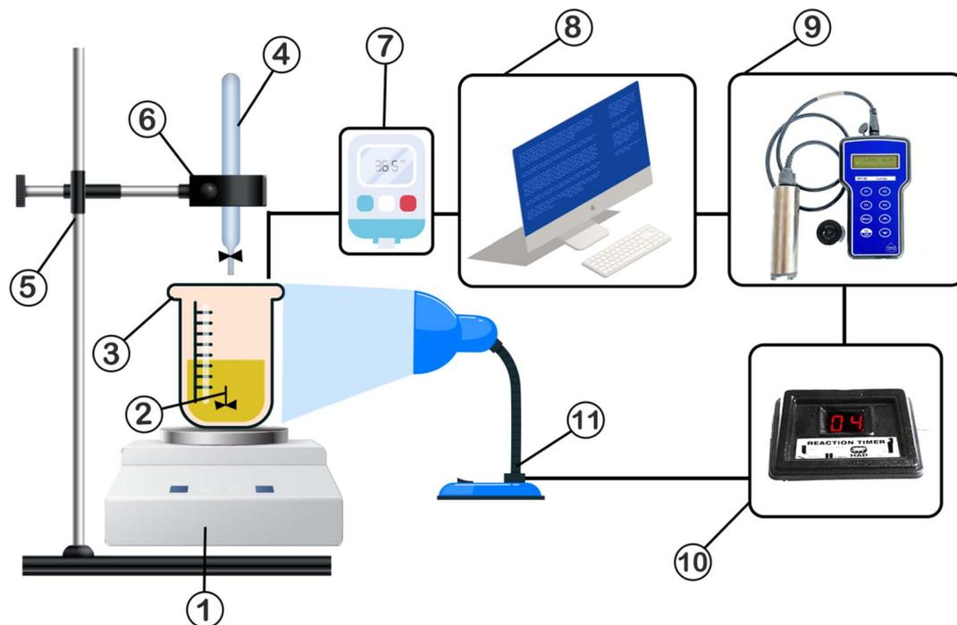
Fig. 1 Schematic diagram of the used laboratory setup ((1) stirrer, (2) mixer or (magnetic stirrer), (3) crystallizer, (4) buret, (5) base, (6) laboratory clamp, (7) thermometer, (8) Pc lab, (9) *in situ* turbidimeter, (10) reaction timer and (11) LED).
