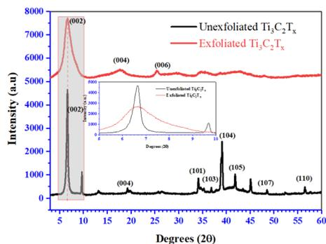
Fig. 5 Unexfoliated and exfoliated  $\text{Ti}_3\text{C}_2\text{T}_x$  XRD patterns.
