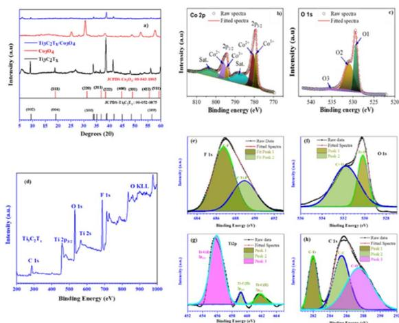
Fig. 6 (a) XRD patterns of  $\text{Ti}_3\text{C}_2\text{T}_x$ ,  $\text{Co}_3\text{O}_4$  NPs, and the  $\text{Ti}_3\text{C}_2\text{T}_x/\text{Co}_3\text{O}_4$  hybrid composite, (b) and (c) XPS spectra of  $\text{Co}_3\text{O}_4$  core levels, (d), (e)–(h) XPS survey and core level spectra of F 1s, O 1s, Ti 2p and C 1s respectively.
