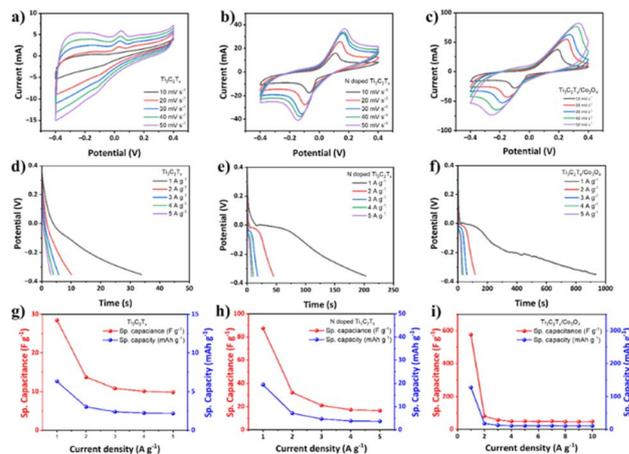
Fig. 7 (a)–(c) CV curves of different electrodes at 10 mV s<sup>-1</sup> scan rate, (d)–(f) discharge curves of different electrodes from GCD analysis at 1 A g<sup>-1</sup> current density, and (g)–(i) specific capacity and specific capacitance in terms of area and mass.
