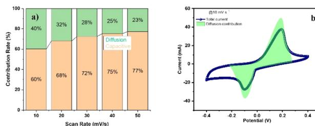
Fig. 8 (a) Contribution ratios of capacitances from the pseudocapacitive controlled reaction and diffusion-controlled reaction at scan rates of 10 to 50  $mV s^{-1}$  and (b) the kinetic analysis of the pseudocapacitive and diffusion parts at a scan rate of 10  $mV s^{-1}$ .
