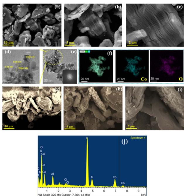
Fig. 4 (a)–(c) FE-SEM images of  $\text{Ti}_3\text{C}_2\text{T}_x$ , (d) HRTEM micrograph of  $\text{Co}_3\text{O}_4$  NPs, (e) TEM image of  $\text{Co}_3\text{O}_4$  NPs with the corresponding FFT shown in the inset, (f) HAADF-EDS color mapping of Co NPs showing Co and O elements, (g)–(i) FE-SEM images of the  $\text{Ti}_3\text{C}_2\text{T}_x/\text{Co}_3\text{O}_4$  hybrid composite, (j) EDS analysis of the  $\text{Ti}_3\text{C}_2\text{T}_x/\text{Co}_3\text{O}_4$  hybrid composite.
