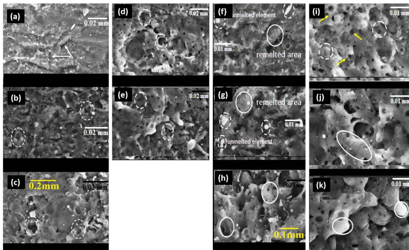
Fig. 3 Top-view SEM images of the samples treated with (a) 3, (b) 5, (c) 7, (d) 9, and (e) 13 laser pulses at a magnification of 1000 $\times$ , and (f) 3, (g) 5, (h) 7, (i) 9, (j) 11, and (k) 13 laser pulses at a magnification power of 2000 $\times$ .
