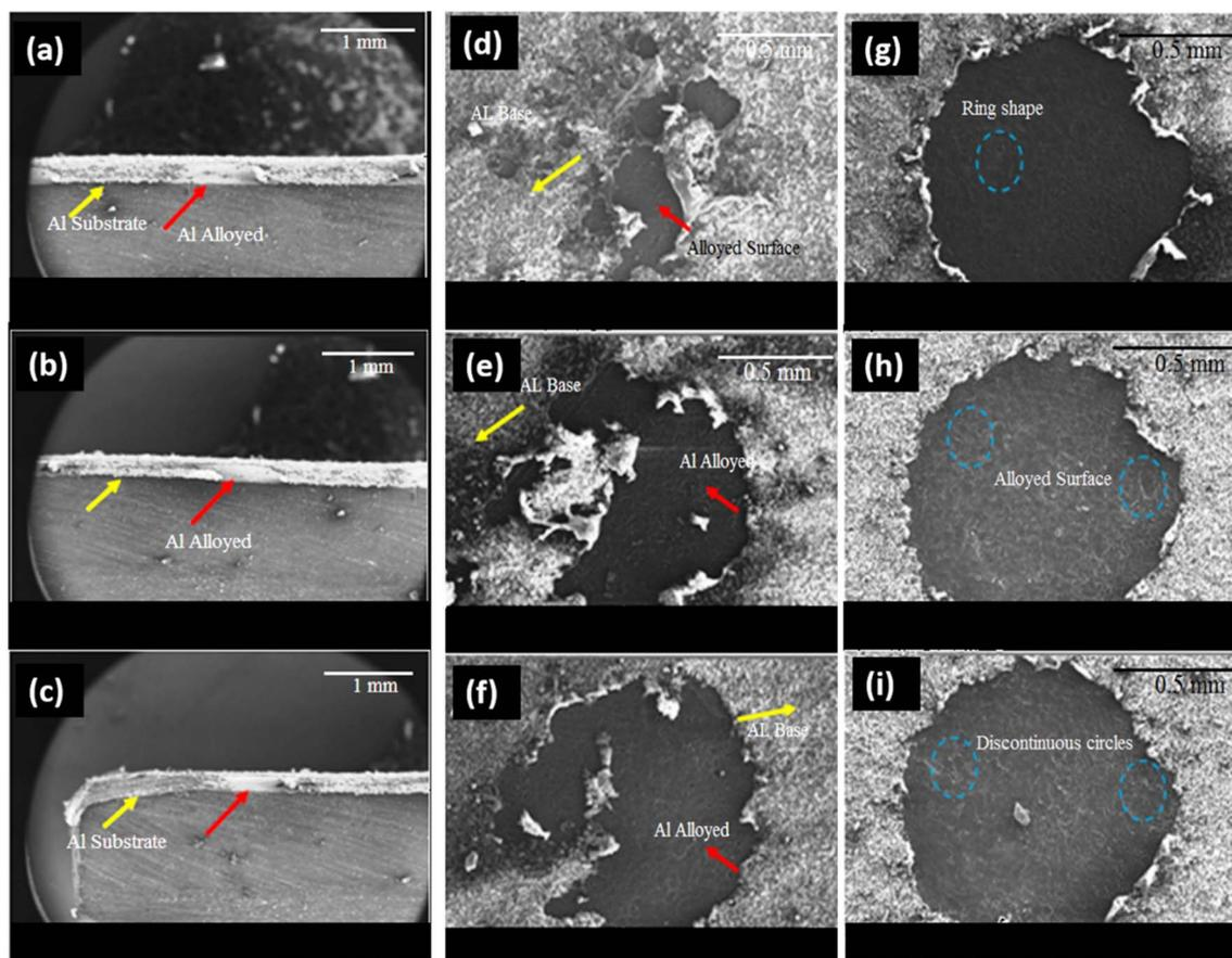
Fig. 2 SEM images showing cross-sectional views of the sample treated at different laser pulses: (a) 3, (b) 5, and (c) 7 pulses with a magnification of 25 $\times$ , and (d–f) the corresponding top-views of the sample with a magnification of 70 $\times$  (red arrow: Al substrate; yellow arrow: alloyed region). (g–i) Top-views of the sample treated at (g) 9, (h) 11, and (i) 13 pulses with a magnification of 70 $\times$ .
