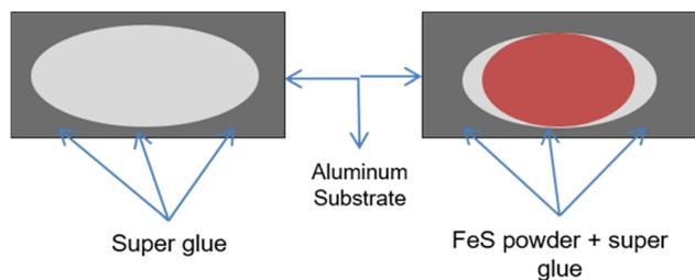
Fig. 1 Configuration of the Fe–SiC coated aluminum substrate.
