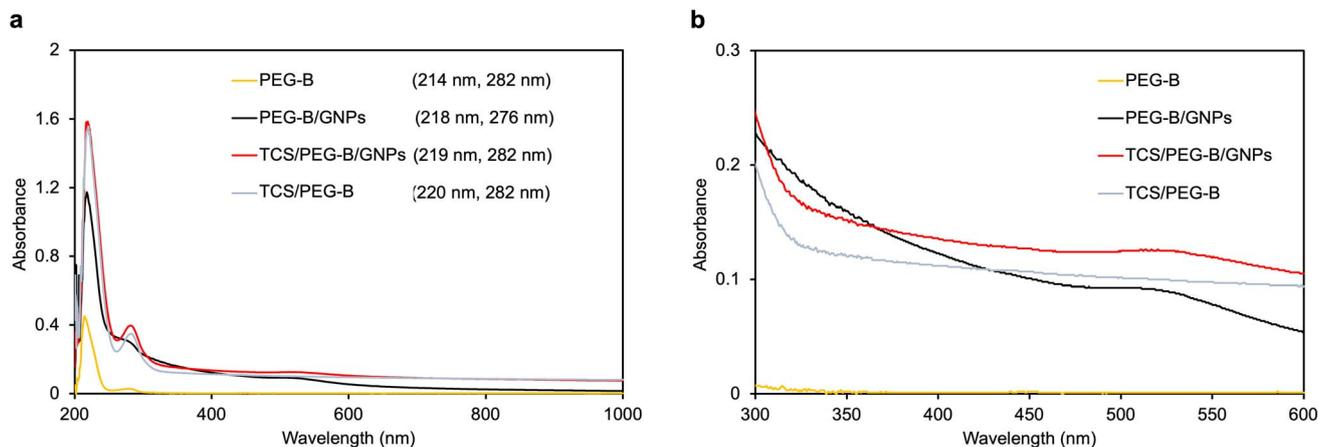
Fig. 2 (a) Absorption spectra of PEG-B, PEG-B/GNPs, TCS/PEG-B/GNPs, and TCS/PEG-B and (b) the absorption spectra of the same samples at wavelengths ranging from 300–600 nm. The peaks of GNPs appear in PEG-B/GNPs and TCS/PEG-B/GNPs.
