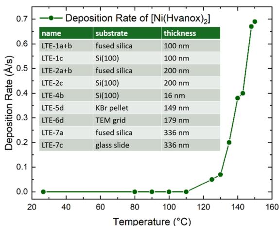
Fig. 1 Temperature-dependent deposition rate of  $[\text{Ni}(\text{Hvanox})_2]$  at a deposition pressure of  $1 \times 10^{-4}$  Pa measured by a QCM sensor; inset: prepared samples including thicknesses.
