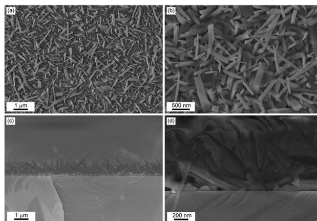
Fig. 9 Top: Representative SEM images (secondary electrons) of a 200 nm [Ni(Hvanox)<sub>2</sub>] film deposited on Si(100) with different magnifications: (a) and (b); Bottom: cross-section view using different magnifications: (c) and (d).
