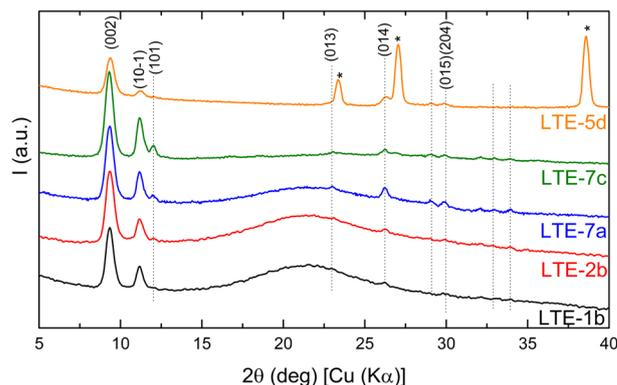
Fig. 3  $\theta/2\theta$  scans of the sample set, displayed on a quadratic scale, with patterns vertically shifted for clarity. Peaks are indexed by their  $(hkl)$  indices, except for those generated by the convolution of three or more reflections. Peaks corresponding to the KBr phase are marked with a star. The dotted vertical lines are a visual aid.
