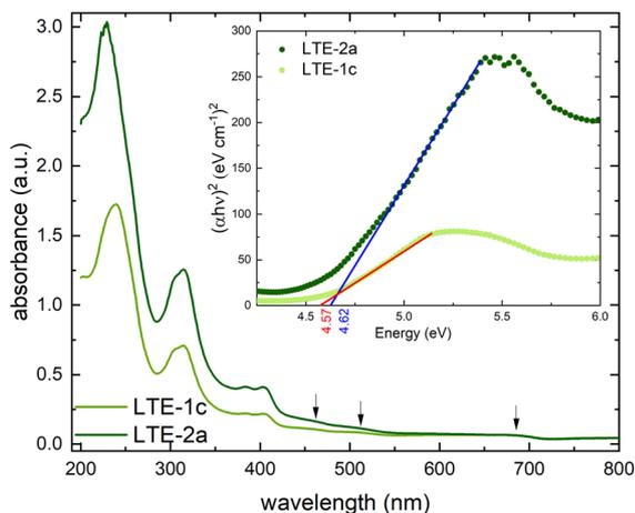
Fig. 2 Solid state electronic absorbance spectra of the 100 nm (pale green) and 200 nm (dark green) thin films of  $[\text{Ni}(\text{Hvanox})_2]$  deposited on fused silica recorded between 800–190 nm. (d–d-transitions highlighted by arrows); inset: determination of the optical band gap for both thin films.
