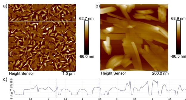
Fig. 6 AFM micrographs of the 16 nm thin film (top; a and b) deposited on Si(100) using different magnifications (a) and (b); the scanned area in (a):  $5 \mu\text{m} \times 5 \mu\text{m}$  with a lateral resolution of  $512 \times 512$  points<sup>2</sup>; (bottom; c) the height indicator profile along the line indicated in (a).
