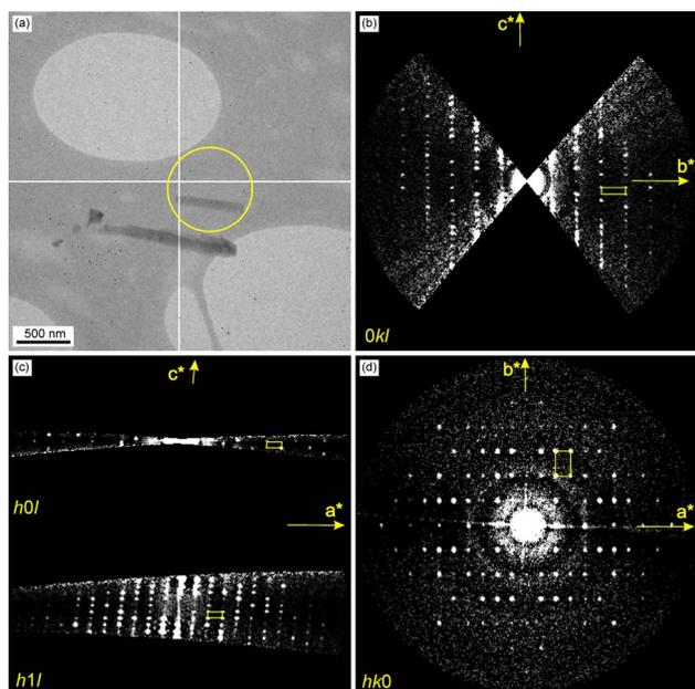
Fig. 10 Electron diffraction results. (a) Image of crystals (crystal used for 3D ED experiment is shown in the yellow circle), (b)  $0kl$  section through the 3D ED data set, (c)  $h0l$  and  $h1l$  sections through the 3D ED data set documenting the extinction rule for  $n$ -glide plane perpendicular to  $b$ -axis ( $h + l = 2n + 1$ ), (d)  $hk0$  section through the 3D ED data set. Yellow parallelepiped shows the corresponding projection of the unit cell.
