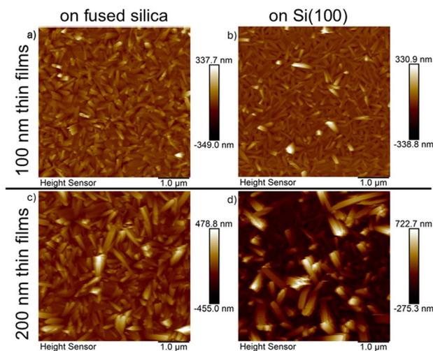
Fig. 5 AFM micrographs (area:  $5 \mu\text{m} \times 5 \mu\text{m}$ ) of the 100 nm thin films (top; a and b) and 200 nm thin films (bottom; c and d) deposited on fused silica (left; a and c) and on Si(100) (right; b and d) using a lateral resolution of  $512 \times 512$  points<sup>2</sup>.
