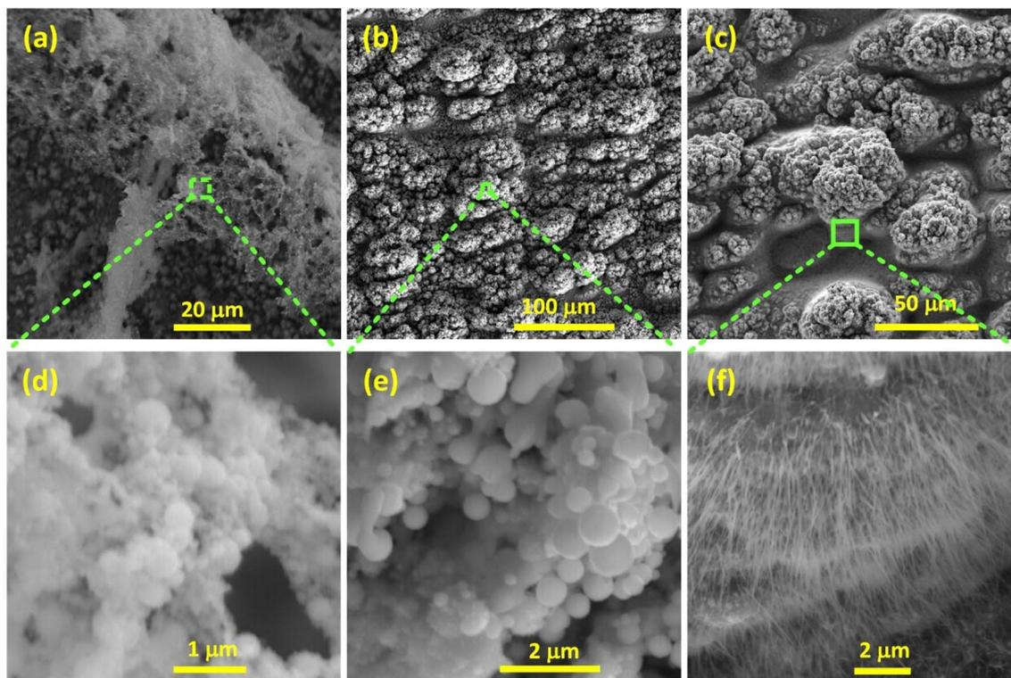
**Fig. 3** (a–c) SEM micrographs of femtosecond laser-structured Cu (20  $\mu\text{m}$  parallel line spacing), with (d–f) corresponding zoomed-in views. (a–d) Cu structured in Ar, showing spherical submicron and nanoparticles. (b–e) Cu structured in air, showing spherical submicron and nanoparticles. (c–f) Cu structured in air and annealed at 350  $^{\circ}\text{C}$ , depicting nanowire-decorated microfeatures.
