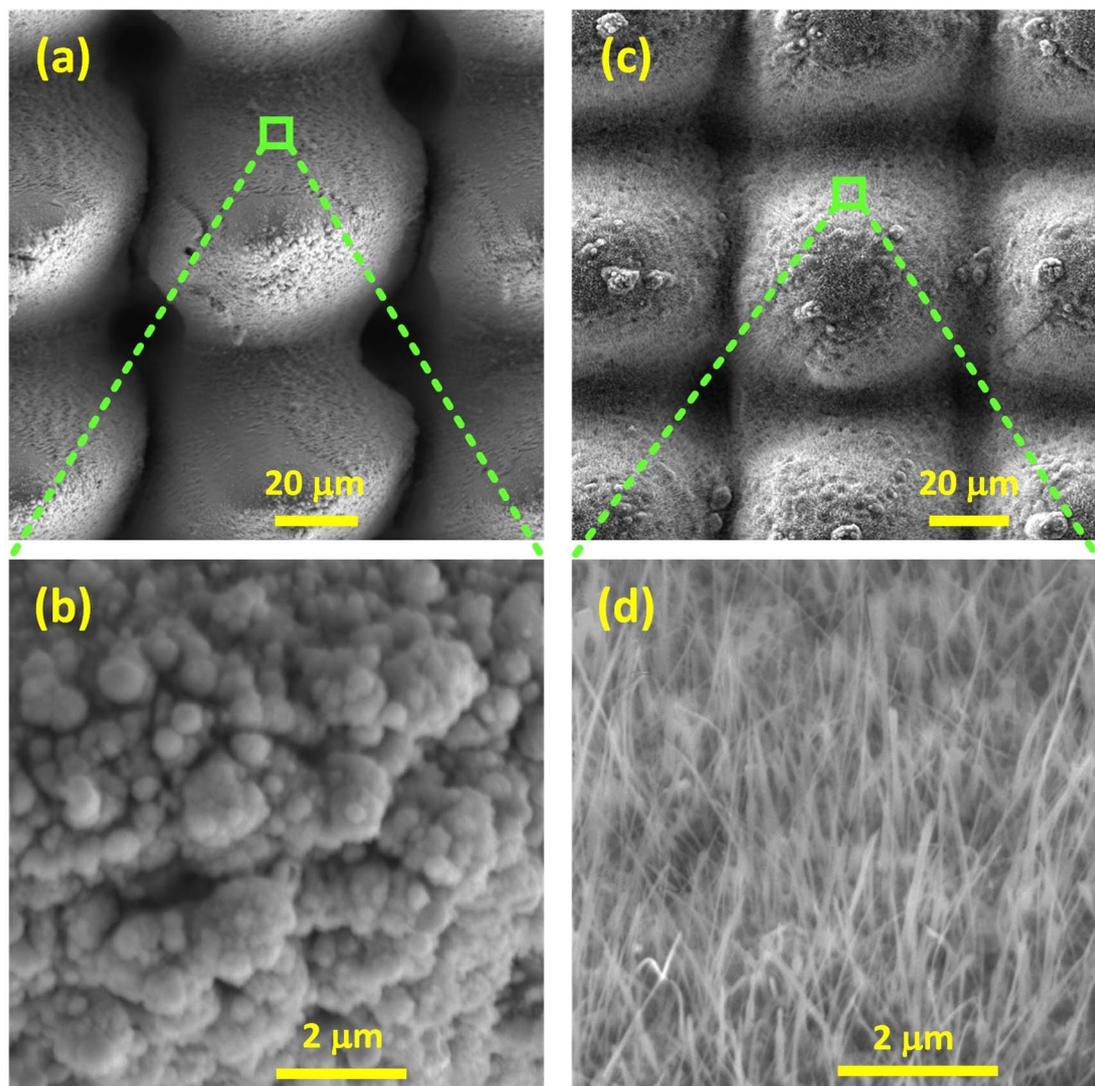
Fig. 4 SEM micrographs of femtosecond laser structured Cu (70  $\mu\text{m}$  crosshatch line spacing) with (a and b) no thermal treatment depicting submicron and nanospheres decorating microdomes, and (c and d) thermally treated at 350  $^{\circ}\text{C}$  in air, showing nanowires decorating the microdomes.
