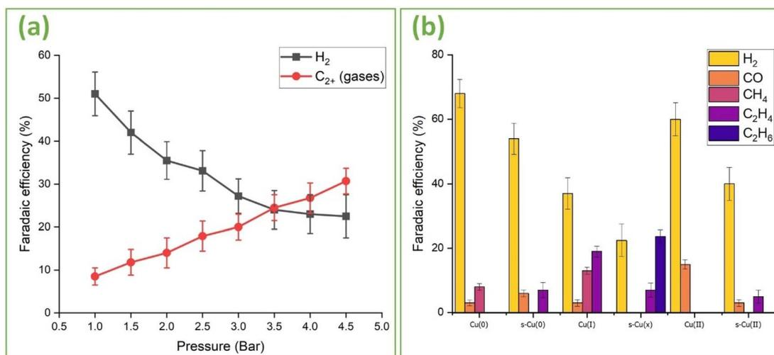
Fig. 8 (a) Faradaic efficiency of  $s\text{-Cu}(x)$  for  $\text{H}_2$  and  $\text{C}_{2+}$  gases as a function of vessel pressure. (b) Faradaic efficiency of all gaseous products observed for unstructured and hierarchically structured  $\text{Cu}(0)$ ,  $\text{Cu}(x)$ , and  $\text{Cu}(\text{II})$  electrodes, respectively.
