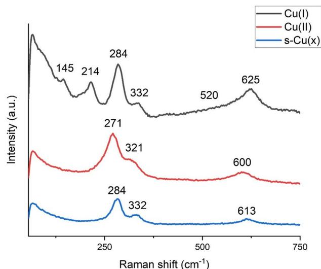
Fig. 5 Raman shift analysis of samples predominantly composed of  $\text{Cu}_2\text{O}$ , as Cu(I), CuO, as Cu(II), and laser structured Cu with mixed oxidation states, s-Cu(x).
