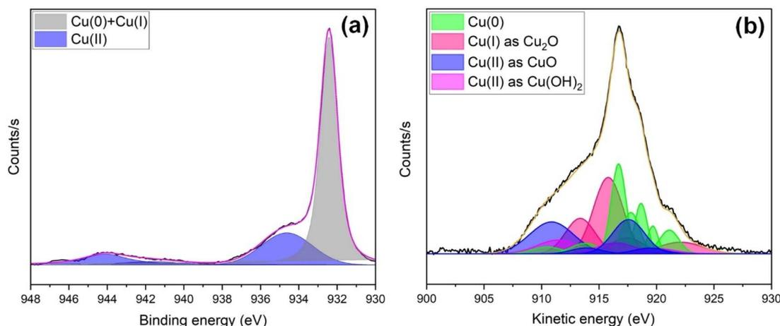
Fig. 7 High-resolution XPS spectra of s-Cu(x) obtained after electrochemical CO<sub>2</sub> reduction, presenting (a) Cu 2p<sub>3/2</sub> and (b) Cu LMM Auger spectral analysis.
