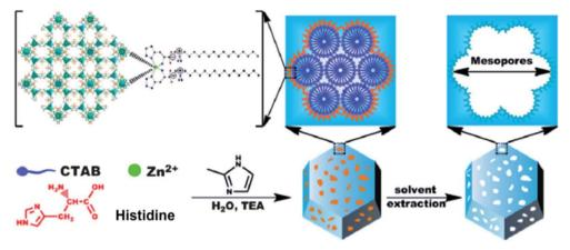
Fig. 6 Possible role of CTAB surfactant and L-histidine co-template in the formation of mesoporous ZIF-8 crystals. This figure has been reproduced from ref. 69 with permission from Royal Society of Chemistry, copyright 2014.
