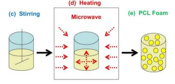
Fig. 3 A real photograph of a microwave oven (a) and a cylindrical mould reactor (b). The processes of stirring (c), microwave heating (d) and the formation of a biodegradable shape memory crosslinked-polycaprolactone (PCL) foam (e). This figure has been reproduced from ref. 54 with permission from Springer Nature copyright 2015.
