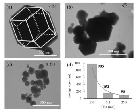
Fig. 7 The shape and size of ZIF-8 crystals synthesized upon addition of triethylamine at various equivalent Zn<sup>2+</sup> ratios: (a) 2.6 mol; (b) 5.1 mol; (c) 25.5 mol. (d) Average particle size of ZIF-8. This figure has been reproduced from ref. 28 with permission from Elsevier, copyright 2017.
