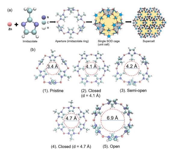
Fig. 5 (a) The structural and topological simulation of ZIF-8 and (b) five different aperture structures of ZIF-8. This figure has been reproduced from ref. 64 with permission from Elsevier, copyright 2021.
