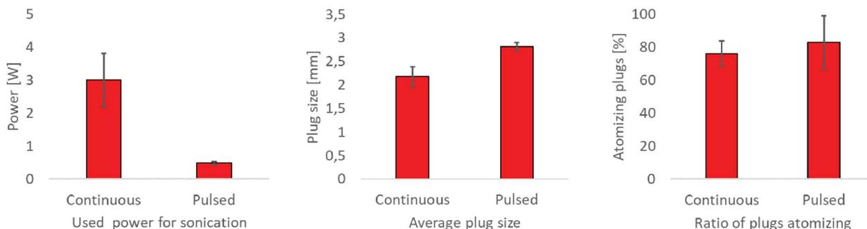
Fig. 5 Comparison of continuous and pulsed sonication.
