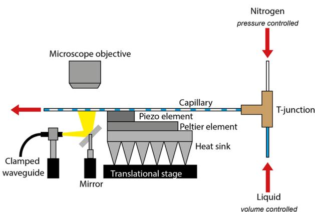
Fig. 1 Schematic of the atomization analysis setup.
