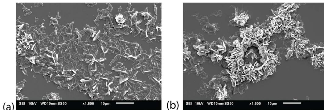
Fig. 8 SEM pictures of dried trimyristine particles. (a) showing singular platelets, while (b) shows a tight agglomerate of platelets.
