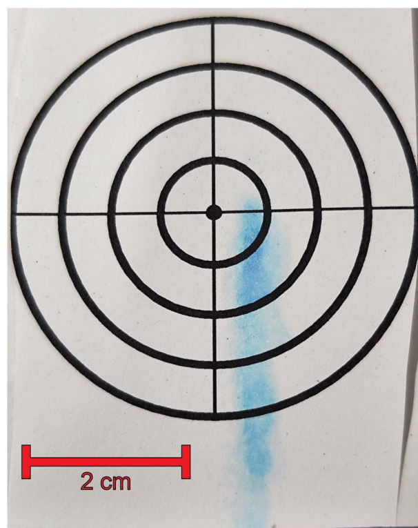
Fig. 7 Spray pattern visualized using a paper in the containment chamber.
