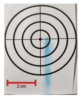
Fig. 7 Spray pattern visualized using a paper in the containment chamber.
