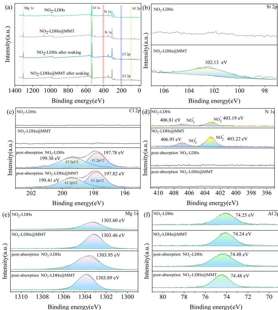
Fig. 7 XPS spectra: (a) survey spectra, (c) Cl 2p, (d) N 1s, (e) Mg 1s, and (f) Al 2p spectra of NO<sub>2</sub>-LDHs and NO<sub>2</sub>-LDHs@MMT before and after adsorption of chlorine ions in simulated concrete pore solutions, and (b) Si 2p spectra of NO<sub>2</sub>-LDHs and NO<sub>2</sub>-LDHs@MMT.
