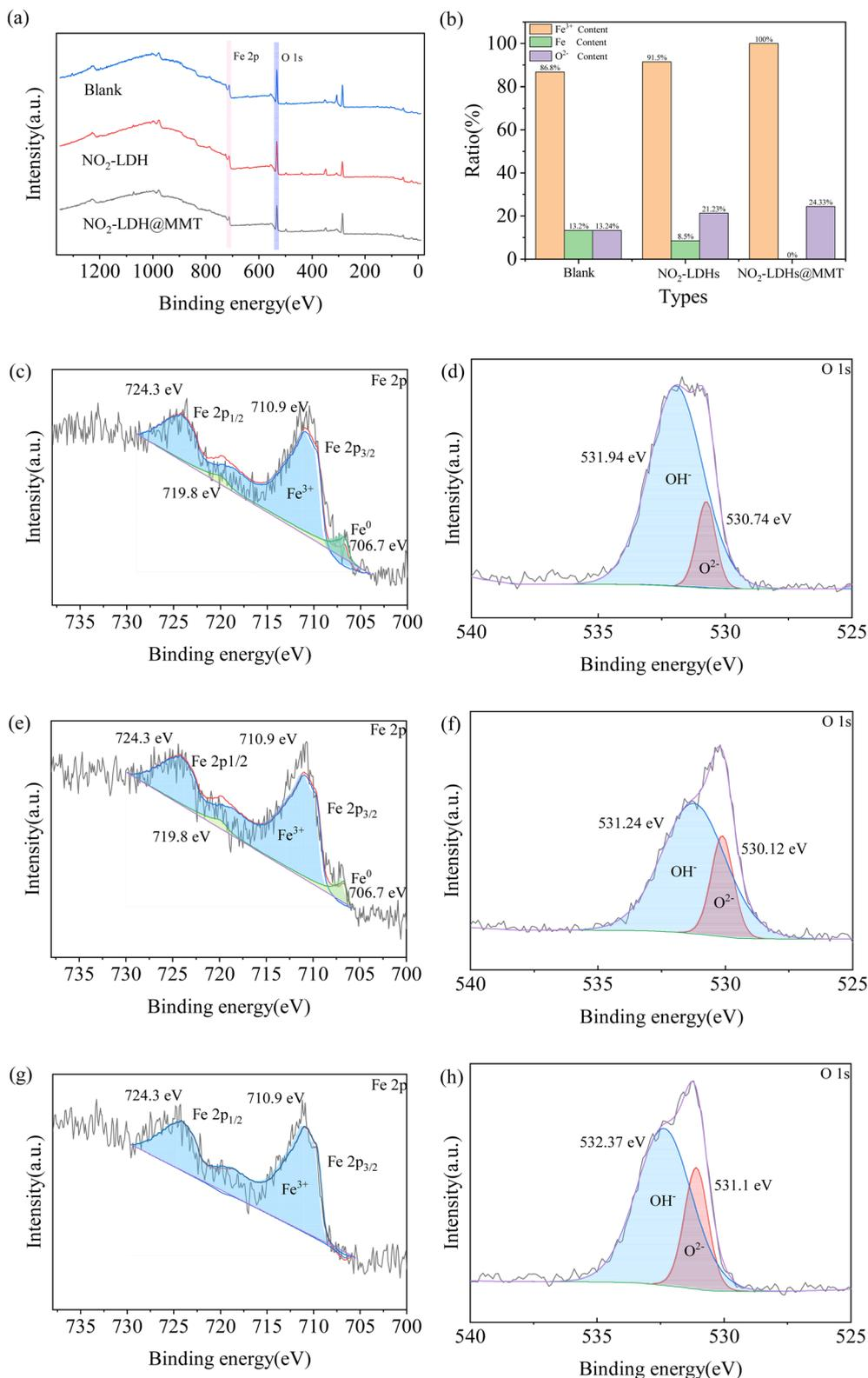
Fig. 15 XPS of rebar electrodes immersed in Ca(OH)<sub>2</sub> passivated for 7 d containing (c and d) blank; (e and f) 1 g L<sup>-1</sup> NO<sub>2</sub>-LDHs; (g and h) 1 g L<sup>-1</sup> NO<sub>2</sub>-LDHs@MMT (a) full and high-resolution spectra; (b) Fe<sup>3+</sup> vs. O<sup>2-</sup> content calculated from XPS results.
