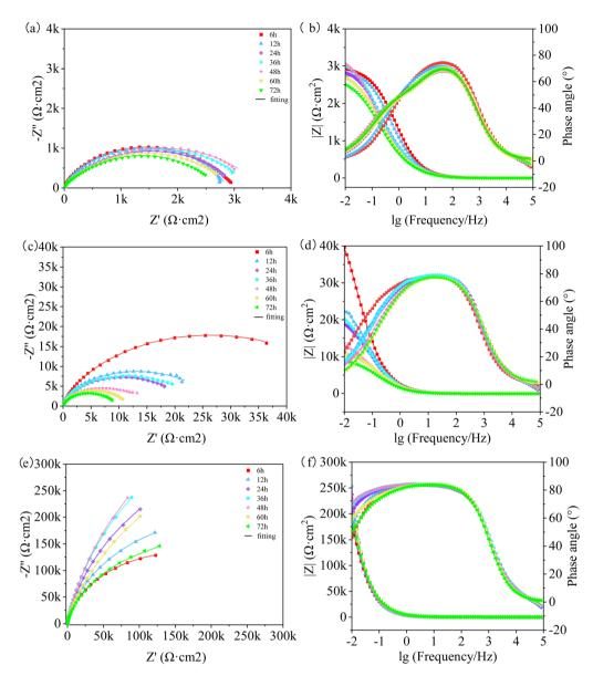
Fig. 12 Nyquist and Bode plots of Q235 steel samples in simulated concrete pore solutions with addition of blank (a, b),  $NO_2$ -LDHs (c, d) and  $NO_2$ -LDHs@MMT (e, f) during 72 h.
