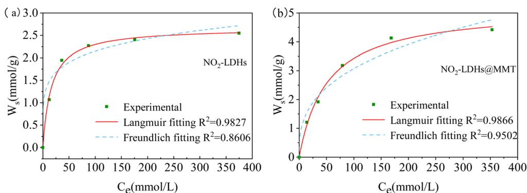
Fig. 10 (a) NO<sub>2</sub>-LDHs and (b) NO<sub>2</sub>-LDHs@MMT isotherm adsorption curves of chloride ions in simulated concrete pore solutions.
