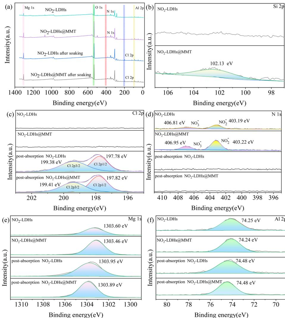
Fig. 7 XPS spectra: (a) survey spectra, (c) Cl 2p, (d) N 1s, (e) Mg 1s, and (f) Al 2p spectra of  $\text{NO}_2$ -LDHs and  $\text{NO}_2$ -LDHs@MMT before and after adsorption of chlorine ions in simulated concrete pore solutions, and (b) Si 2p spectra of  $\text{NO}_2$ -LDHs and  $\text{NO}_2$ -LDHs@MMT.
