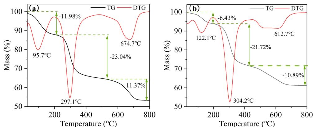
Fig. 8 TG-DTG patterns of the synthesized NO<sub>2</sub>-LDHs (a) and NO<sub>2</sub>-LDHs@MMT (b).
