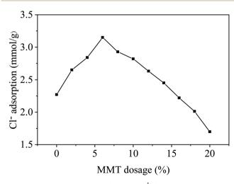
Fig. 2 Adsorption of Cl $^-$  in 100 mmol L $^{-1}$  Cl $^-$  solution by the synthesised NO $_2$ -LDHs@MMT with different MMT doping levels.
