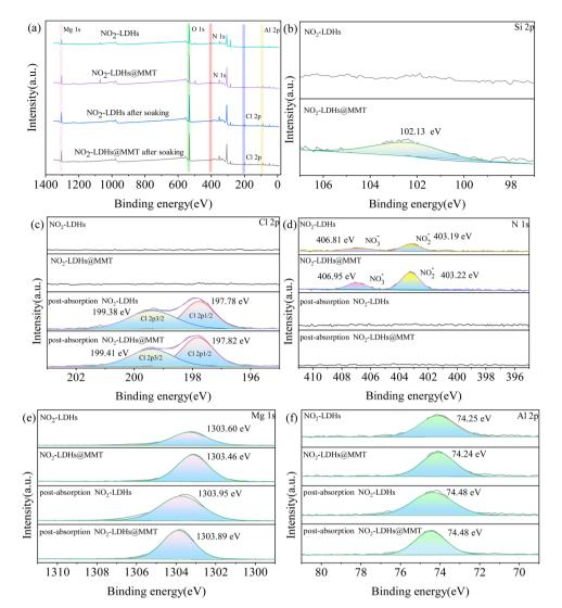
Fig. 7 XPS spectra: (a) survey spectra, (c) Cl 2p, (d) N 1s, (e) Mg 1s, and (f) Al 2p spectra of  $NO_2$ -LDHs and  $NO_2$ -LDHs@MMT before and after adsorption of chlorine ions in simulated concrete pore solutions, and (b) Si 2p spectra of  $NO_2$ -LDHs and  $NO_2$ -LDHs@MMT.
