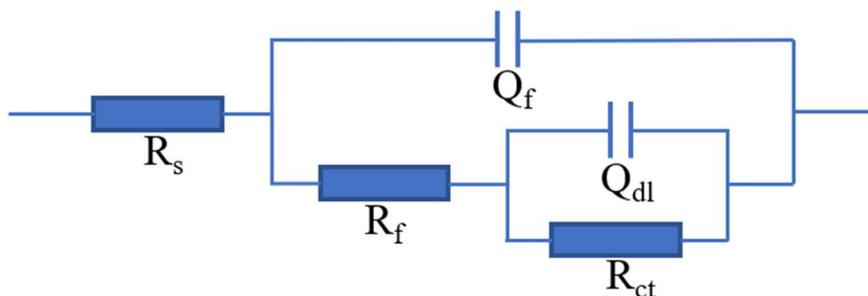
Fig. 13 The equivalent circuit for analyzing EIS data.
