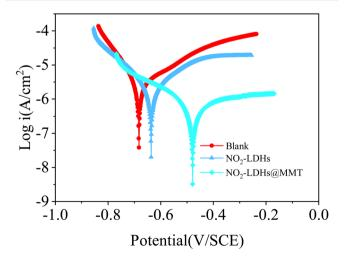
Fig. 14 Tafel curve of carbon steels in simulated concrete pore solutions with addition of NO $_2$ -LDHs@MMT, NO $_2$ -LDHs and blank (after soaking in simulated concrete pore solutions and with addition of NO $_2$ -LDHs@MMT, NO $_2$ -LDHs and blank for 72 h).
