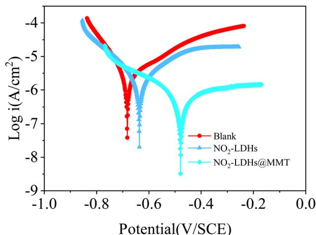
Fig. 14 Tafel curve of carbon steels in simulated concrete pore solutions with addition of NO<sub>2</sub>-LDHs@MMT, NO<sub>2</sub>-LDHs and blank (after soaking in simulated concrete pore solutions and with addition of NO<sub>2</sub>-LDHs@MMT, NO<sub>2</sub>-LDHs and blank for 72 h).
