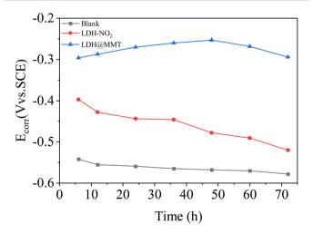
Fig. 11 Change in the corrosion potential ( $E_{corr}$ ) of steel samples in different corrosion solutions over 72 h.
