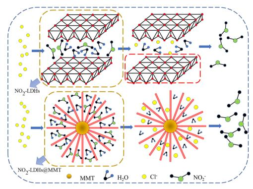
Fig. 16 Schematic diagram of NO<sub>2</sub> and Cl displacement in composite NO<sub>2</sub>-LDHs@MMT
