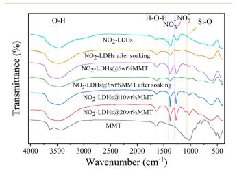
Fig. 4 FTIR patterns of MMT, NO<sub>2</sub>-LDHs and NO<sub>2</sub>-LDHs@MMT before and after 2 h adsorption in simulated concrete pore solutions
