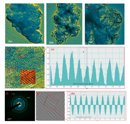
Fig. 6 (a) TEM images of NO<sub>2</sub>-LDHs; (b and c) TEM images of NO<sub>2</sub>-LDHs@MMT; (d) HRTEM image of NO<sub>2</sub>-LDHs@MMT; (e) plot profile of HRTEM lattice fringes of NO2-LDHs@MMT; (f) FFT pattern of NO2-LDHs@MMT; (g) IFFT pattern of NO2-LDHs@MMT; (h) plot profile of IFFT pattern lattice fringes of NO2-LDHs@MMT.
