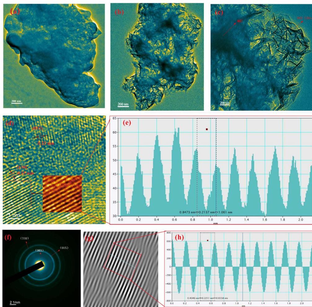
**Fig. 6** (a) TEM images of  $\text{NO}_2$ -LDHs; (b and c) TEM images of  $\text{NO}_2$ -LDHs@MMT; (d) HRTEM image of  $\text{NO}_2$ -LDHs@MMT; (e) plot profile of HRTEM lattice fringes of  $\text{NO}_2$ -LDHs@MMT; (f) FFT pattern of  $\text{NO}_2$ -LDHs@MMT; (g) IFFT pattern of  $\text{NO}_2$ -LDHs@MMT; (h) plot profile of IFFT pattern lattice fringes of  $\text{NO}_2$ -LDHs@MMT.
