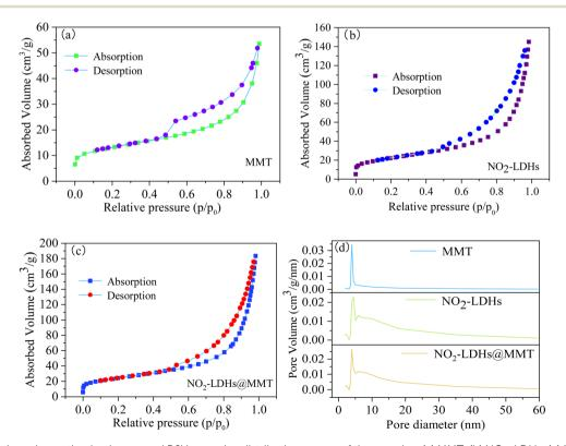
Fig. 9 N<sub>2</sub> adsorption—desorption isotherms and BJH pore size distribution curves of the samples: (a) MMT, (b) NO<sub>2</sub>-LDHs, (c) NO<sub>2</sub>-LDHs@MMT and (d) pore size distribution curves of samples.
