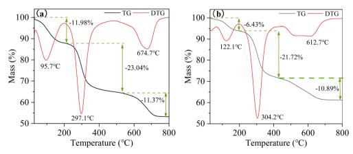
Fig. 8 TG-DTG patterns of the synthesized NO<sub>2</sub>-LDHs (a) and NO<sub>2</sub>-LDHs@MMT (b).
