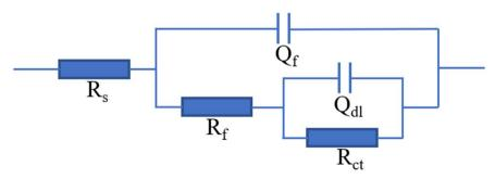
Fig. 13 The equivalent circuit for analyzing EIS data.
