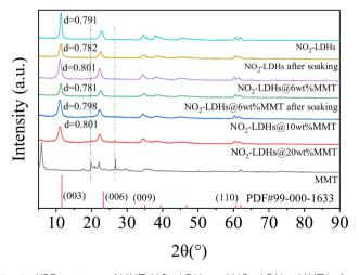
Fig. 3  $\,$  XRD patterns of MMT, NO<sub>2</sub>-LDHs and NO<sub>2</sub>-LDHs@MMT before and after 2 h adsorption in simulated concrete pore solutions.
