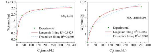
Fig. 10 (a) NO<sub>2</sub>-LDHs and (b) NO<sub>2</sub>-LDHs@MMT isotherm adsorption curves of chlorine ions in s simulated concrete pore solutions.
