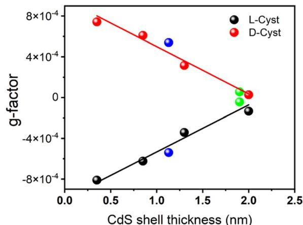
Fig. 10 Variation of the CD *g*-factor of the DRs with their shell thickness (Table S4†). Green dots: additional data from ref. 16 (Tables S2 and S3†) and blue ones from ref. 34 with identical seed diameter.
