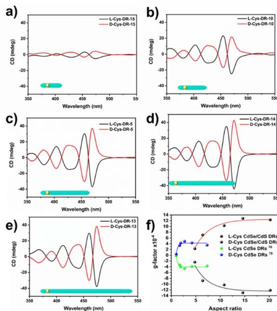
Fig. 11 Variation of the CD signal with the DR aspect ratio, in the 400–500 nm region of the CdS absorption (CdSe seed size  $D_s = 3.2$  nm). (a–e) CD signal of DR-15, DR-10, DR-5, DR-14, and DR-13, from Table 3; (f) Resulting CD *g*-factor variation of the same DRs (lines are guides for the eyes). Blue and green data are from ref. 78 for pure CdSe QRs. Lines are also guides for the eyes.
