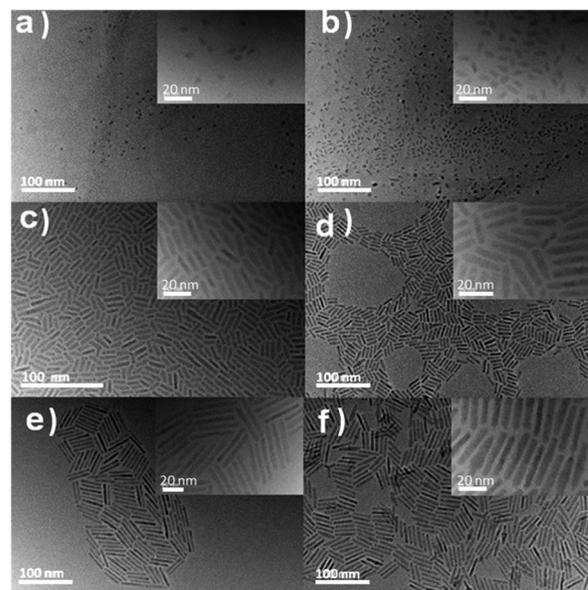
Fig. 2 TEM images of DRs (DR-1 to DR-6) synthesized under different reaction times starting with the same CdSe seed solution ( $D_s = 3.2$  nm) at a concentration of 14  $\mu\text{M}$ . (a) 30 s, (b) 60 s, (c) 120 s, (d) 240 s, (e) 480 s, and (f) 960 s.
