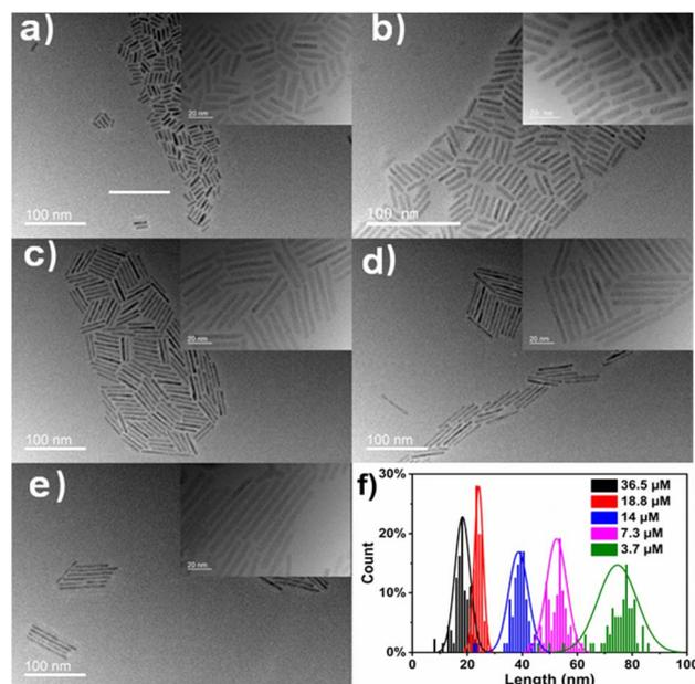
**Fig. 6** TEM images of DRs synthesized starting with different CdSe seed concentrations. (a) DR-15, 36.5  $\mu$ M, (b) DR-10, 18.8  $\mu$ M, (c) DR-5, 14  $\mu$ M, (d) DR-14, 7.3  $\mu$ M, and (e) DR-13, 3.7  $\mu$ M, and (f) variation of DR length distributions obtained at different seed concentrations (593 K).
