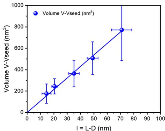
Fig. 7 Linear variation of the volume  $V - V_s$  of the DRs versus the length  $l = L - D$  of their cylindrical part in the 1D-growth regime, at  $T = 593$  K and after 8 min of reaction, when varying the seed concentration [CdSe].
