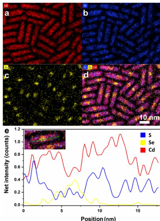
Fig. 4 Representative TEM EDS mapping of one of the many samples, DR15, with a length of  $18.3 \pm 2.8$  nm and a diameter of  $3.8 \pm 0.6$ : [(a–c) representative EDS mapping images for Cd, S, and Se, (d) merging of Cd, S, and Se maps, and (e) line-scan distribution profiles of Cd, S, and S in a DR.
