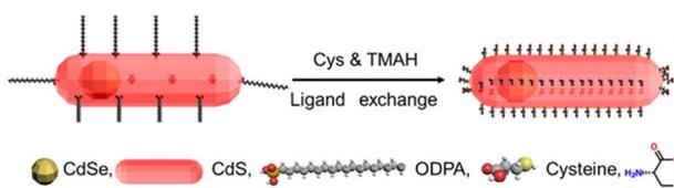
Fig. 8 The ligand exchange process of DRs from the oil phase to the aqueous phase.
