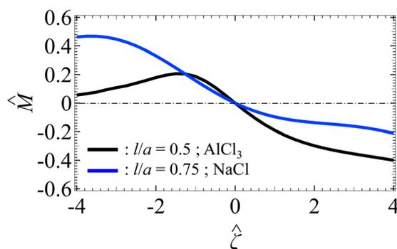
Fig. 4 The non-dimensionalized diffusio-phoretic mobility  $\hat{M}$  versus the non-dimensionalized colloid surface potential  $\hat{\zeta}$  in different porous media saturated with different electrolyte solutions of ionic strength  $I = 0.25$  mM. Black line: a denser porous medium (the ratio of the screening length to the colloid radius  $l/a = 0.5$ ) saturated with a  $\text{AlCl}_3$  solution. Blue line: a less dense porous medium ( $l/a = 0.75$ ) saturated with a  $\text{NaCl}$  solution.
