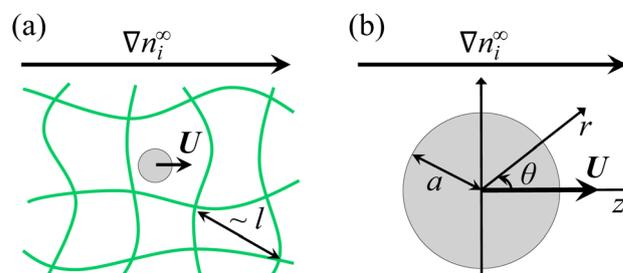
Fig. 1 A concentration gradient of a mixture of  $N$  ionic species,  $\nabla n_i^\infty$  with  $i = 1, 2, \dots, N$ , induces the diffusiophoretic motion of a colloid of radius  $a$  in a static porous medium with a constant screening length  $l$ . The colloid diffusiophoretic velocity  $U$  is parallel to  $\nabla n_i^\infty$ . (a) A wholistic view of the colloid and the porous medium. (b) The adopted spherical coordinate and moving reference frame.
