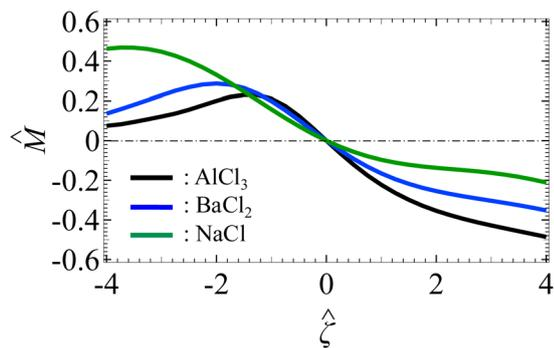
Fig. 3 The non-dimensionalized diffusio-phoretic mobility  $\hat{M}$  versus the non-dimensionalized colloid surface potential  $\hat{\zeta}$  in the same porous media (the ratio of the screening length to the colloid radius  $l/a = 0.75$ ) saturated with different electrolyte solutions of ionic strength  $I = 0.25$  mM. Black line:  $\text{AlCl}_3$ . Blue line:  $\text{BaCl}_2$ . Green line:  $\text{NaCl}$ .
