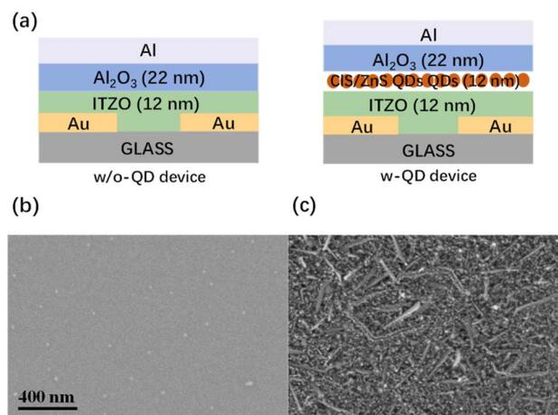
Fig. 2 (a) Schematic of the device structures. SEM images of Al<sub>2</sub>O<sub>3</sub> (b) and QDs films (c).
