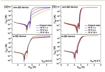
Fig. 5 Transfer characteristics of TFTs after NBS (a) and PBS (b). The transfer curves were recorded after applying gate bias stresses denoted in the figures.
