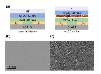
Fig. 2 (a) Schematic of the device structures. SEM images of  $Al_2O_3$  (b) and QDs films (c).
