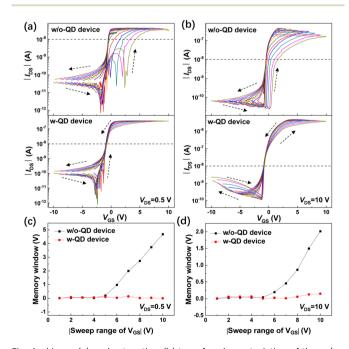
Fig. 4 Linear (a) and saturation (b) transfer characteristics of the w/o-QD and w-QD devices. The dashed lines indicate the level of  $I_{\rm DS}$  at which the memory window value is extracted; memory windows extracted from the linear (c) and saturation (d) transfer curves.
