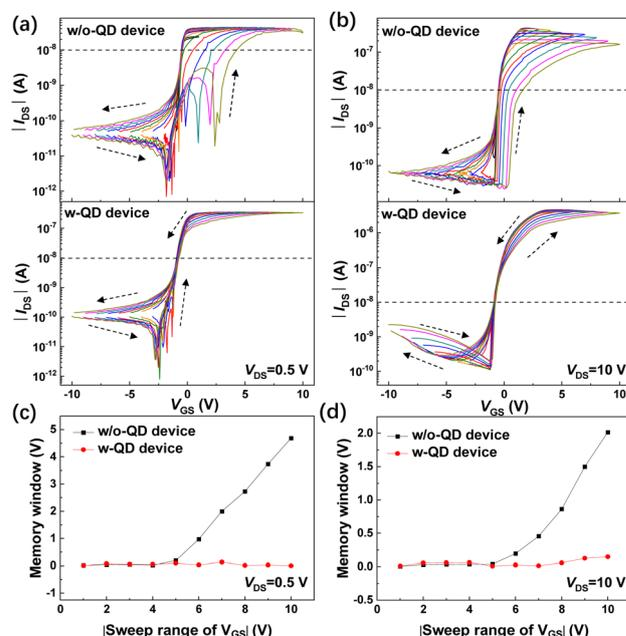
Fig. 4 Linear (a) and saturation (b) transfer characteristics of the w/o-QD and w-QD devices. The dashed lines indicate the level of  $I_{\text{DS}}$  at which the memory window value is extracted; memory windows extracted from the linear (c) and saturation (d) transfer curves.
