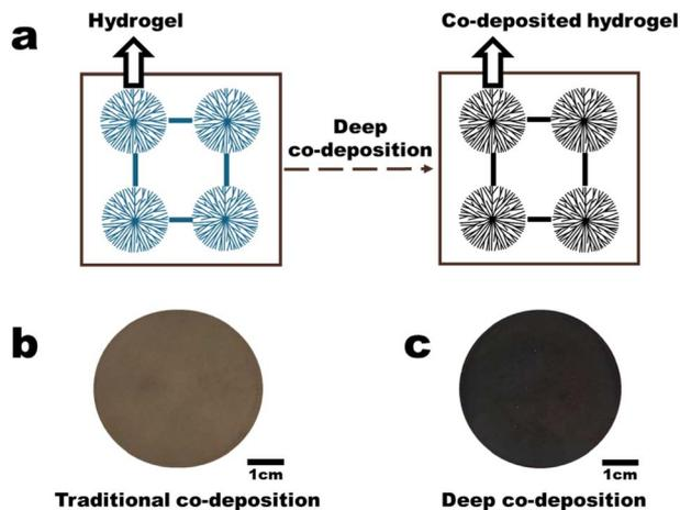
**Fig. 1** (a) Schematic illustration of the deep co-deposition method; (b) digital image of a traditional co-deposited PVDF membrane under one solar illumination of  $1 \text{ kW m}^{-2}$  (wet state); (c) digital image of a deep co-deposited PVDF membrane under a solar illumination of  $1 \text{ kW m}^{-2}$  (wet state).
