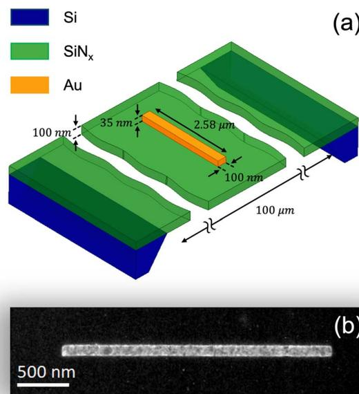
Fig. 3 Fabrication details of the plasmonic dipole antenna. (a) Schematic of the fabrication stack-up, showing the dipole dimensions (length =  $2.58 \mu\text{m}$ , width =  $100 \mu\text{m}$ , thickness =  $35 \text{ nm}$ ) and the suspended membrane ( $100 \mu\text{m} \times 100 \mu\text{m}$ , thickness =  $100 \text{ nm}$ ) supported by a silicon substrate. (b) High-angle annular dark-field scanning transmission electron microscopy (HAADF-STEM) image of the fabricated plasmonic dipole.
