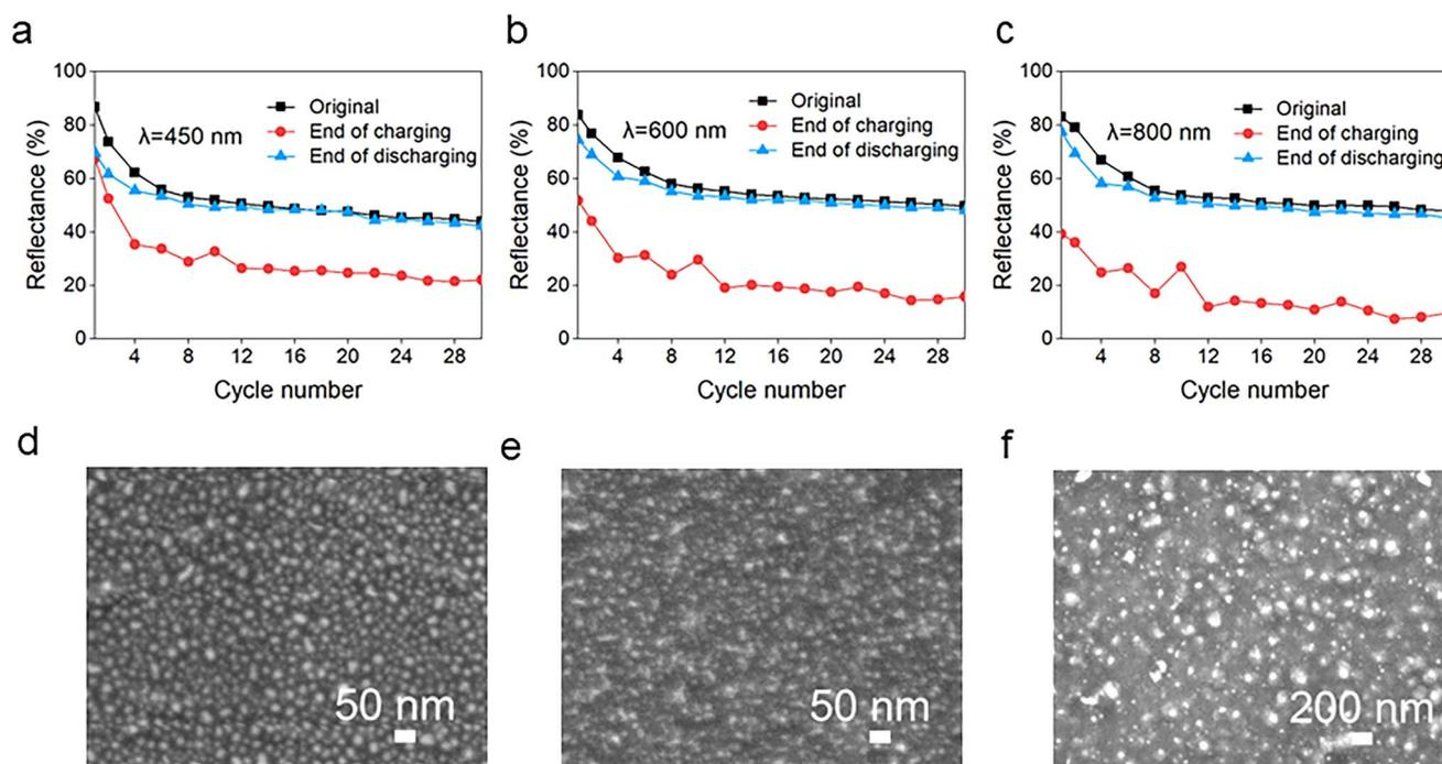
Fig. 4 Cycling performance of the absorber. (a–c) *In situ* reflectance spectrum corresponding to three states (original, end of charge, end of discharge) at different wavelengths ((a)  $\lambda = 450$  nm, (b)  $\lambda = 600$  nm, (c)  $\lambda = 800$  nm) during cycling. (d–f) SEM images of the anode after the 2nd cycle, the 15th cycle and the 25th cycle.
