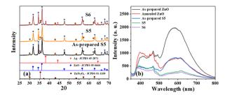
Fig. 1 (a) XRD patterns of as-prepared S5, S5, and S6, which matched the standard JCPDS cards of Ag, ZnO, and ZnFe<sub>2</sub>O<sub>4</sub>, (b) photo-luminescence spectra of as-prepared ZnO, ZnO annealed at 350 °C for 4 h, and as-prepared S5, S5, and S6.
