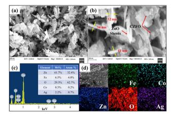
Fig. 2 FESEM images of S6 at (a) 90 KX magnification, (b) 300 KX magnification, (c) EDS spectra; inset table shows the elemental composition, and (d) elemental mapping of Fe, Co, Zn, O, and Aq.
