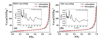
Fig. 4 (a)  $N_2$  adsorption—desorption isotherms for S5 and (b) S6; insets show the respective BJH plots.
