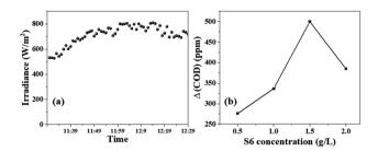
Fig. 7 (a) Solar irradiance measured during the photocatalysis from 11:30 am to 12:30 pm, plot of (b) change in the COD of ciprofloxacin solution versus \$6 concentration under 60 min sunlight exposure.
