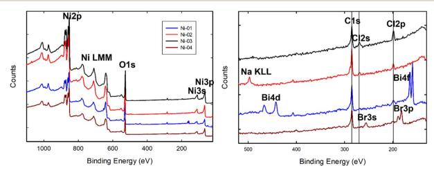
Fig. 1 Survey spectra for commercial samples of unmodified NiO nanoparticles from four different suppliers. The energy region between 520 and 130 eV is magnified at right to show the peaks assigned to various impurities present on the different samples
