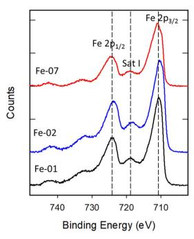
Fig. 7 High resolution spectra of Fe 2p region after Shirley background subtraction for three Fe<sub>2</sub>O<sub>3</sub> nanomaterials.
