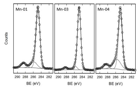
Fig. 5 High resolution spectra of the C 1s region for three Mn<sub>2</sub>O<sub>3</sub> samples. Fits are shown by the solid grey (components) and black (sum) lines.
