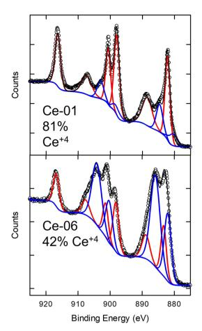
Fig. 8 High resolution spectra of Ce 3d region for two different  $CeO_2$  nanoparticles. The hollow circles are the experimental data points while the solid black line represents the total fit to the data which is a sum of the contributions of two different oxidation states, represented by the red (+4) and blue (+3) lines.
