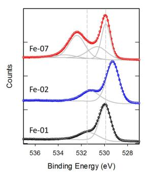
Fig. 4 High resolution spectra of the O 1s region for three different  $Fe_2O_3$  nanoparticle samples. Fits are shown by the solid grey lines with the overall fit shown by the solid black, blue and red lines.
