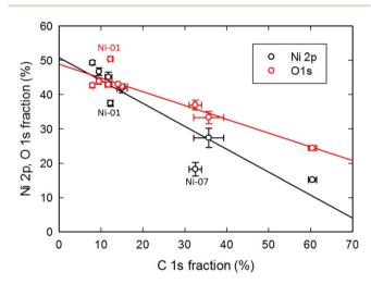
Fig. 3 Correlation of Ni 2p and O 1s signal intensities with the C 1s signal (based on the HR data) for the eight NiO samples. Outlier points are labelled and discussed in the text.
