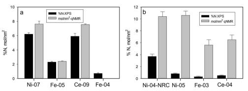
Fig. 10 Comparison of %N measured by XPS with molecules per nm<sup>2</sup> from qNMR for (a) aminated and (b) PVP modified metal oxide NPs. The qNMR signal for Fe-04 was weak and not quantified.
