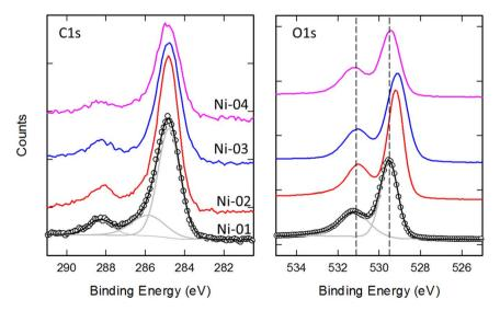
Fig. 2 High resolution spectra of the C 1s and O 1s regions for four unmodified NiO nanoparticle samples. Fits to the Ni-01 spectra are shown by the solid grey (components) and black (sum) lines.
