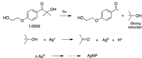
**Scheme 1** Norrish type I cleavage of I-2959 following UV photoexcitation and a subsequent PCET reaction between the ketyl radical and a silver cation to form one equivalent of reduced silver that spontaneously aggregates to form AgNPs.
