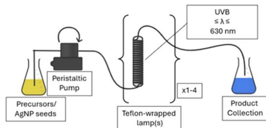
**Fig. 1** Generalized diagram of the photochemical flow setup utilized in this study. The identity of each lamp varied depending on the desired outcome, with UVB being used to generate AgNP seeds from a precursor solution and visible LEDs of varying wavelengths to transform seeds into d and tAgNPs. A photograph of the true system is available in the ESI (Fig. S6).†
