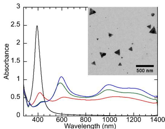
Fig. 5 UV-vis-NIR absorbance spectra for the slow cyclic flow of AgNP seeds (black) through a series of 4 single wrapped green LEDs ( $\lambda = 522$  nm), with approximate exposure times of 31.3 h (red), 63 h (green), and 72 h (blue). (Inset): the TEM image of the final product from cyclic flow of AgNP seeds through green LEDs, following 72 h of exposure. Contrast and brightness have been adjusted for image clarity. Scale bar: 500 nm. For lamp emission spectra, see Fig. S1.†
