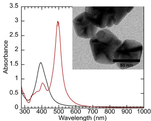
Fig. 4 UV-vis absorbance spectra of a single pass of AgNP seeds through a double-wrapped blue LED ( $\lambda = 455$  nm). The spectrum of initial seeds is shown in black, and the product is shown in red. Residence time was approximately 3.3 hours. (Inset): TEM image of the product from single pass flow of AgNP seeds through a double-wrapped blue LED. Contrast and sharpness have been adjusted for image clarity. Scale bar: 50 nm. For lamp emission spectra, see Fig. S1.†
