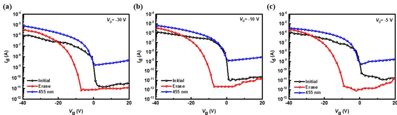
Fig. 7 Transfer characteristics of the hybrid floating-gate photomemory device using ODA-6FDA/PVSK as the floating gate under different  $V_D$  for both reading and photowriting: (a)  $-30$  V, (b)  $-10$  V, and (c)  $-5$  V, with an electrical erasing time of 1 s and a photowriting light intensity of  $12.5$   $\text{mW cm}^{-2}$ . Note that the photowriting was conducted at  $V_G = 0$  V.
