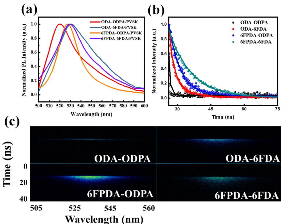
Fig. 2 (a) PL emission spectra, (b) 1D TRPL decaying profiles, and (c) 2D TRPL patterns of the PAA/PVSK thin films excited by using a 375 nm laser source.
