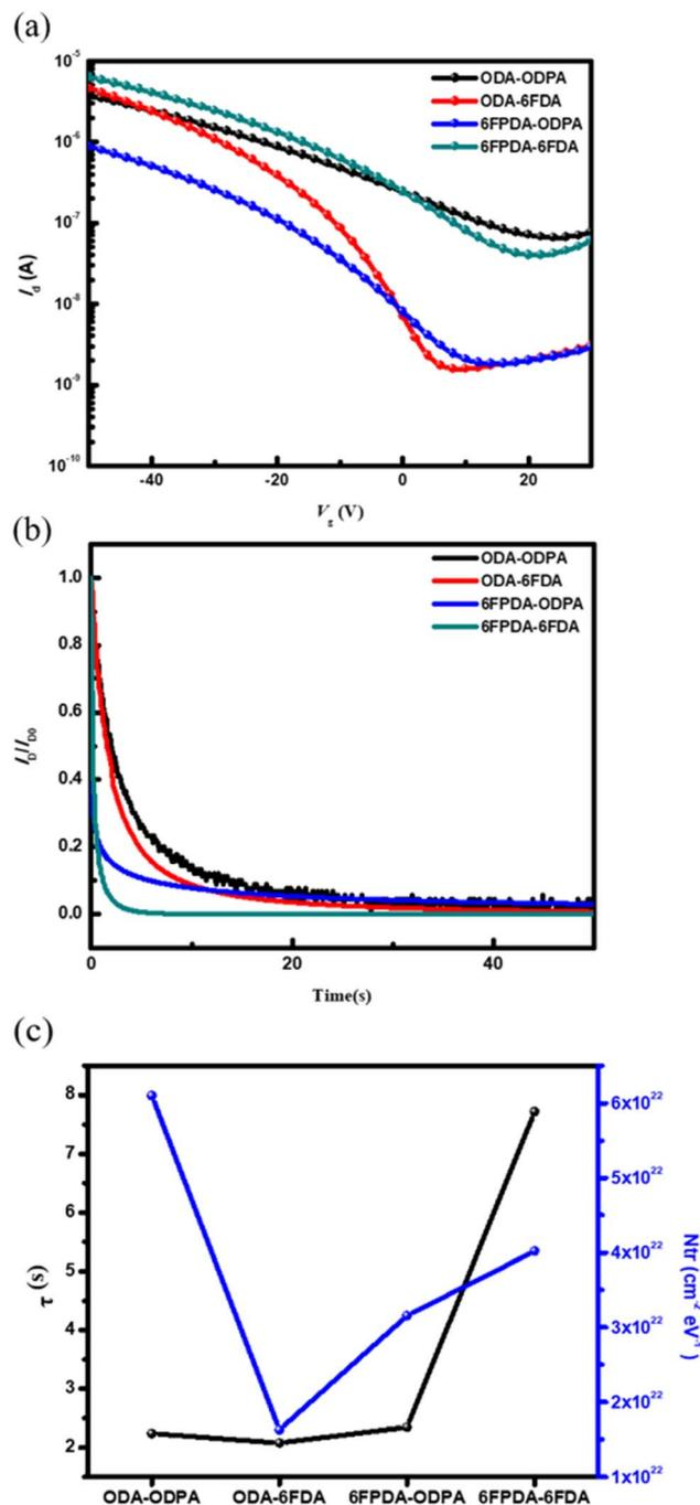
Fig. 4 (a) Transfer curves, (b) bias stress stability test at  $V_D$  and  $V_G = -10$  V, and (c) the characteristic time constant ( $\tau$ ) in the bias stress response and the interfacial trap density ( $N_{tr}$ ) derived from the subthreshold swing (SS) of the transfer curves of the devices comprising pure PAAs/100 nm-thick SiO<sub>2</sub> dielectrics and a pentacene channel. The transfer curves were scanned at a fixed  $V_D = -40$  V from  $V_G = 30$  to  $-50$  V.
