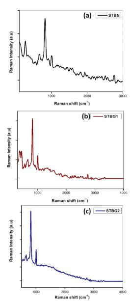
Fig. 8 Raman analysis of (a) STBN, (b) STBG1 and (c) STBG2 composites
