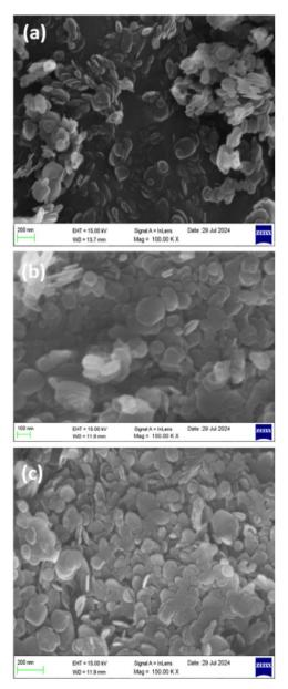
Fig. 7 SEM images of (a) STBN, (b) STBG1 and (c) STBG2 composite.
