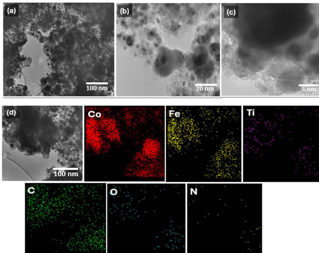
Fig. 3 TEM images of the M3 catalyst (scale bar: (a) 100 nm, (b) 20 nm and (c) 5 nm); (d) elemental mapping of the M3 catalyst.
