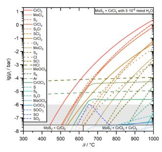
Fig. 1 Calculation results of the temperature-dependent vapor pressures of the dominant vapor species over an equimolar mixture of  $MoS_2$  and  $CrCl_3$  with traces of water. The predicted condensed phases at the bottom are displayed for amounts larger than  $10^{-5}$  mmol. The grey area indicates vapor pressures that are too low to contribute to transport processes.
