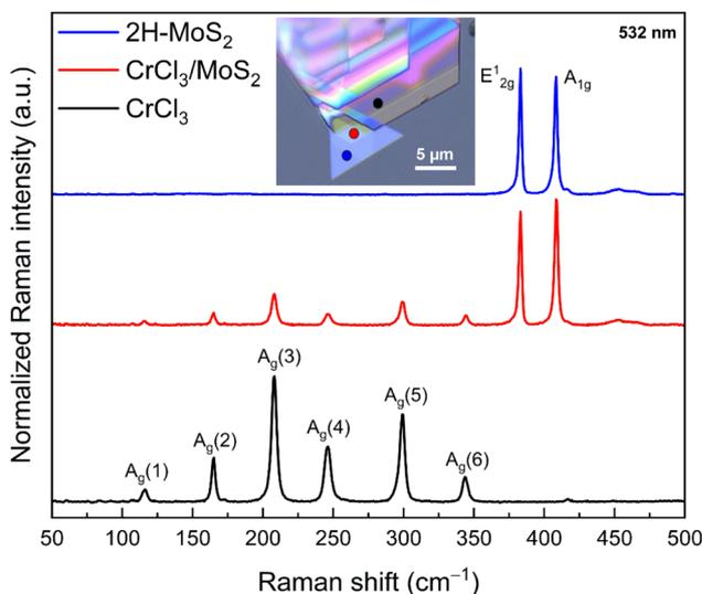
Fig. 6 Raman spectra of the  $\text{CrCl}_3/\text{MoS}_2$  vertical heterostructure. Raman spectra recorded from the three different regions, labelled in the inset optical microscope image of  $\text{CrCl}_3/\text{MoS}_2$ , showing the anti-parallel triangles of  $\text{MoS}_2$  and  $\text{CrCl}_3$  on the top. There are overlapping Raman signatures with  $\text{MoS}_2$  (red line).
