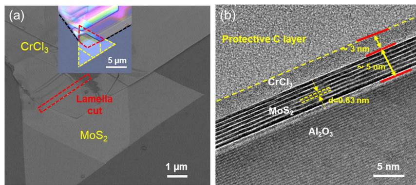
Fig. 7 Structural characterization of the  $\text{CrCl}_3/\text{MoS}_2$  heterostructure. (a) SEM image of the  $\text{CrCl}_3/\text{MoS}_2$  heterostructure, highlighting the marked region for lamella cutting, with the corresponding optical microscope image (inset in (a)). (b) Cross-sectional HRTEM image of a vertically-staked  $\text{CrCl}_3/\text{MoS}_2$  heterostructure. The image shows the distinct layers of  $\text{MoS}_2$  and  $\text{CrCl}_3$ , highlighting their interface and alignment.
