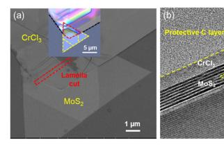
Fig. 7 Structural characterization of the  $CrCl_3/MoS_2$  heterostructure. (a) SEM image of the  $CrCl_3/MoS_2$  heterostructure, highlighting the marked region for lamella cutting, with the corresponding optical microscope image (inset in (a)). (b) Cross-sectional HRTEM image of a vertically-staked  $CrCl_3/MoS_2$  heterostructure. The image shows the distinct layers of  $MoS_2$  and  $CrCl_3$ , highlighting their interface and alignment.
