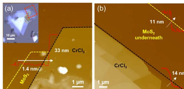
Fig. 5 (a) AFM images of the  $\text{CrCl}_3/\text{MoS}_2$  heterostructure for the marked region in the optical microscope image (inset in (a)). (b) AFM image of another  $\text{CrCl}_3/\text{MoS}_2$  heterostructure. Inset: height profile along the white arrow, shown with the same x-scale as the image scale.
