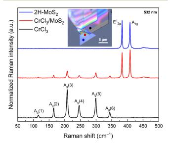
Fig. 6 Raman spectra of the CrCl<sub>3</sub>/MoS<sub>2</sub> vertical heterostructure. Raman spectra recorded from the three different regions, labelled in the inset optical microscope image of CrCl<sub>3</sub>/MoS<sub>2</sub>, showing the antiparallel triangles of MoS<sub>2</sub>, and CrCl<sub>3</sub> on the top. There are overlapping Raman signatures with MoS<sub>2</sub> (red line).
