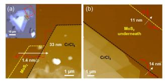
Fig. 5 (a) AFM images of the  $CrCl_3/MoS_2$  heterostructure for the marked region in the optical microscope image (inset in (a)). (b) AFM image of another  $CrCl_3/MoS_2$  heterostructure. Inset: height profile along the white arrow, shown with the same x-scale as the image scale.
