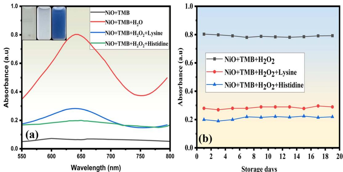
Fig. 3 (a) UV-vis absorption spectra of the NiONPs with and without the addition of histidine and lysine; (b) stability of NiONPs (catalytic activity and POD-like activity).
