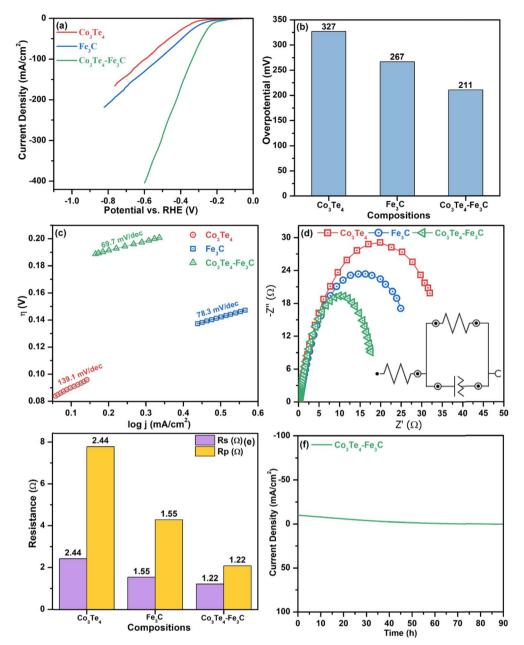
Fig. 5 HER electrocatalysis: (a) LSV curves, (b) bar chart of overpotential at 10 mA cm<sup>-2</sup> current density, (c) Tafel plots, (d) EIS plots, (e) comparison of  $R_p$  and  $R_s$ , and (f) stability (i-t) curve of  $Co_3Te_4$ ,  $Fe_3C$ , and  $Co_3Te_4$ - $Fe_3C$ .
