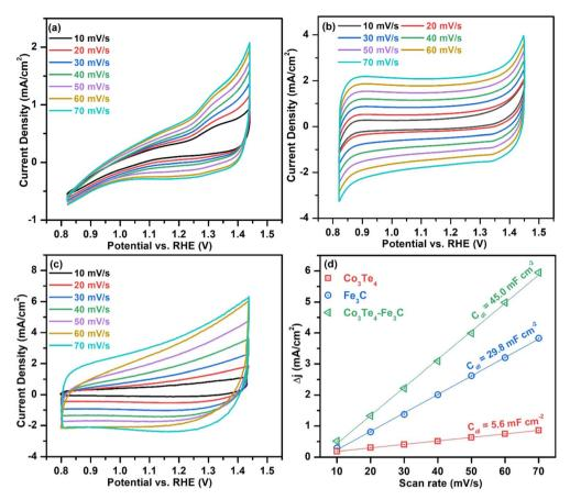
Fig. 6 Cyclic voltammograms without the faradaic zone at 10-70 mV s<sup>-1</sup> for (a) Co<sub>3</sub>Te<sub>4</sub>, (b) Fe<sub>3</sub>C, and (c) Co<sub>3</sub>Te<sub>4</sub>-Fe<sub>3</sub>C, and (d) comparison of  $C_{\rm dl}$  plots for ECSA evaluation.
