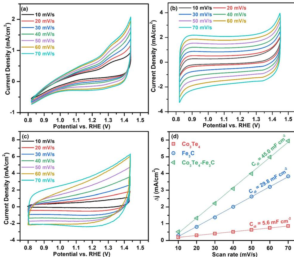
Fig. 6 Cyclic voltammograms without the faradaic zone at 10–70  $\text{mV s}^{-1}$  for (a)  $\text{Co}_3\text{Te}_4$ , (b)  $\text{Fe}_3\text{C}$ , and (c)  $\text{Co}_3\text{Te}_4\text{-Fe}_3\text{C}$ , and (d) comparison of  $C_{\text{dl}}$  plots for ECSA evaluation.
