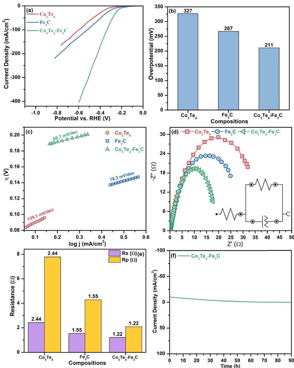
Fig. 5 HER electrocatalysis: (a) LSV curves, (b) bar chart of overpotential at  $10 \text{ mA cm}^{-2}$  current density, (c) Tafel plots, (d) EIS plots, (e) comparison of  $R_p$  and  $R_s$ , and (f) stability ( $i-t$ ) curve of  $\text{Co}_3\text{Te}_4$ ,  $\text{Fe}_3\text{C}$ , and  $\text{Co}_3\text{Te}_4\text{-Fe}_3\text{C}$ .
