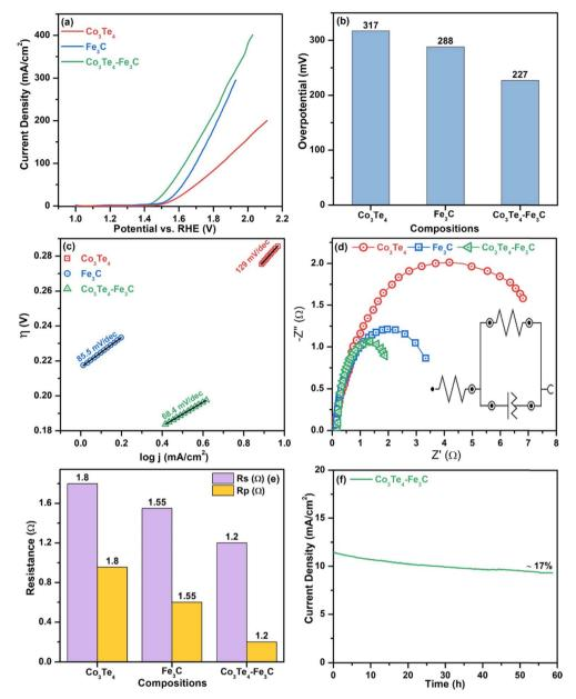
Fig. 4 OER electrocatalysis: (a) LSV curves, (b) bar chart of the overpotential at 10 mA cm<sup>-2</sup> current density, (c) Tafel plots, (d) EIS plots, (e) comparison of  $R_p$  and  $R_s$ , and (f) stability (i-t) curve of  $Co_3Te_4$ ,  $Fe_3C$  and  $Co_3Te_4$ - $Fe_3C$ .
