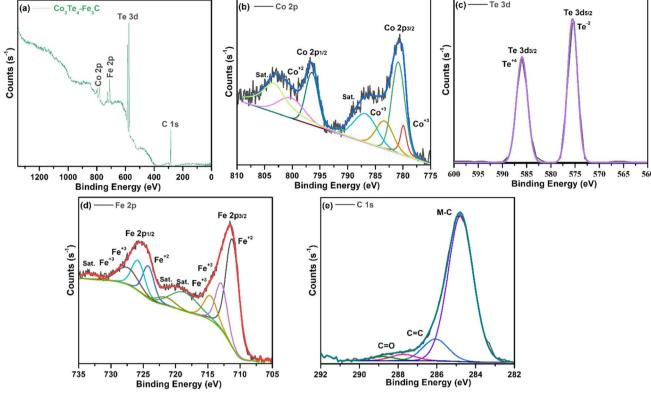
Fig. 2 High resolution XPS spectrum of  $Co_3Te_4$ – $Fe_3C$ : (a) survey spectrum, and deconvoluted curves of (b)  $Co\ 2p$ , (c)  $Te\ 3d$ , (d)  $Fe\ 2p$  and (e)  $C\ 1s$ .
