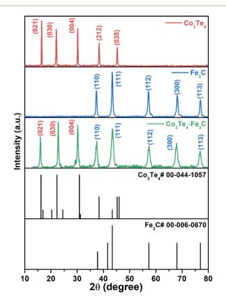
Fig. 1 XRD patterns of as-synthesized Co<sub>3</sub>Te<sub>4</sub>, Fe<sub>3</sub>C, and Co<sub>3</sub>Te<sub>4</sub>-Fe<sub>3</sub>C catalysts.
