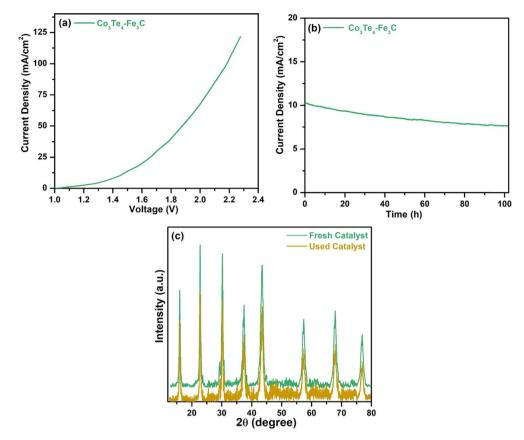
Fig. 7 (a) LSV polarization curve for overall water splitting, (b) chronoamperometric curve of  $Co_3Te_4-Fe_3C$  using an overall two electrode set-up, and (c) XRD pattern of the used catalyst after overall water-splitting.
