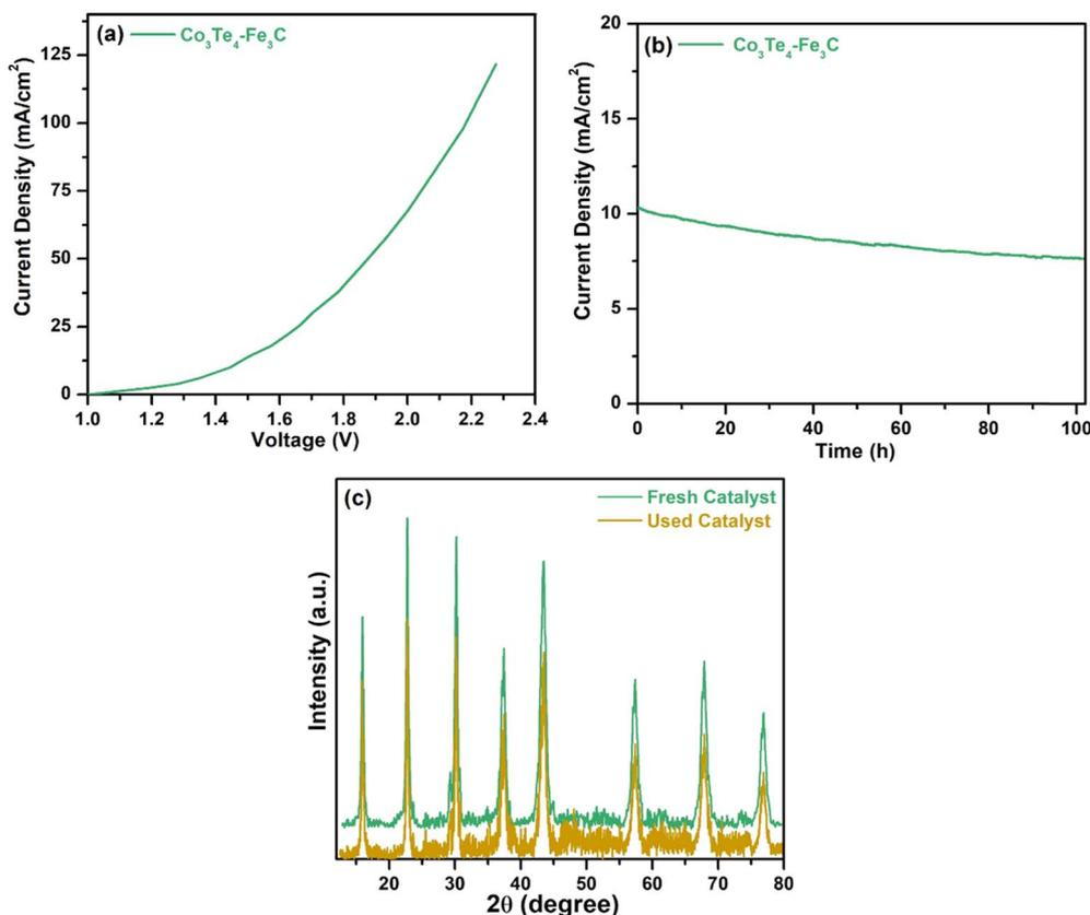
Fig. 7 (a) LSV polarization curve for overall water splitting, (b) chronoamperometric curve of  $\text{Co}_3\text{Te}_4\text{-Fe}_3\text{C}$  using an overall two electrode set-up, and (c) XRD pattern of the used catalyst after overall water-splitting.
