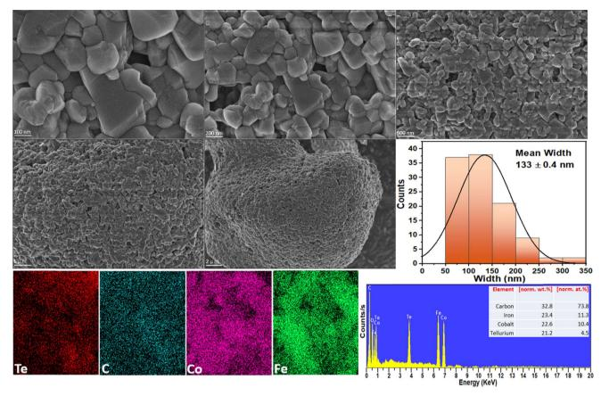
Fig. 3 High and low magnification FE-SEM analysis, and the corresponding widths, and EDX spectrum/mapping of the Co<sub>3</sub>Te<sub>4</sub>−Fe<sub>3</sub>C composite.
