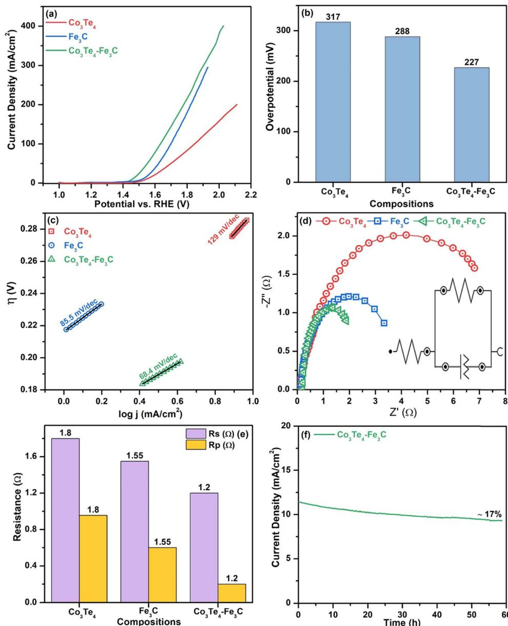
Fig. 4 OER electrocatalysis: (a) LSV curves, (b) bar chart of the overpotential at 10 mA cm<sup>-2</sup> current density, (c) Tafel plots, (d) EIS plots, (e) comparison of  $R_p$  and  $R_s$ , and (f) stability ( $i-t$ ) curve of Co<sub>3</sub>Te<sub>4</sub>, Fe<sub>3</sub>C and Co<sub>3</sub>Te<sub>4</sub>-Fe<sub>3</sub>C.
