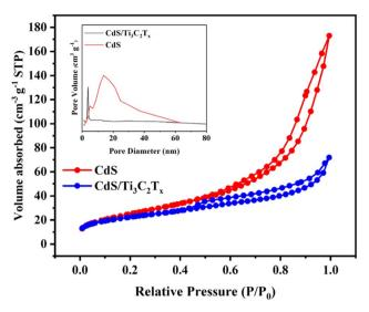
Fig. 6 Nitrogen adsorption–desorption isotherms were conducted for  $Ti_3C_2T_x$  MXene, mesoporous CdS nanoparticles, and the CdS/ $Ti_3C_2T_x$  heterostructure. Pore-size distributions are depicted in the inset.
