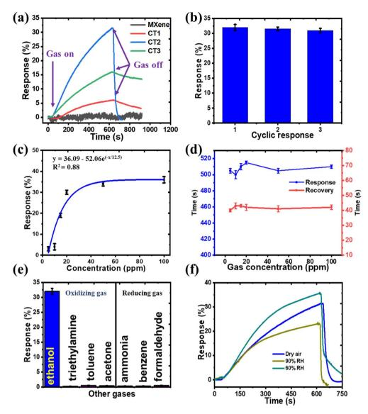
Fig. 7 (a) The response/recovery properties of pristine  $Ti_3C_2T_x$  MXene, and prepared CdS/ $Ti_3C_2T_x$ -based sensors, toward ethanol molecules (20 ppm). (b) Repeatability curve and (c) Langmuir isotherm curve of CT2 responses against different ethanol concentrations, and (d) response and recovery time. Response of the CT2 sensor to (e) several gases (f) at various levels of relative humidity.
