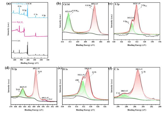
$\textbf{Fig. 5} \quad \textbf{(a) Survey spectra of the mesoporous CdS nanoparticle,} \ \textbf{Ti}_{3}\textbf{C}_{2}\textbf{T}_{x} \ \textbf{MXene, and CdS/Ti}_{3}\textbf{C}_{2}\textbf{T}_{x} \ \textbf{heterostructure.} \ \textbf{XPS spectra of the CdS/Ti}_{3}\textbf{C}_{2}\textbf{T}_{x} \ \textbf{MXene, and CdS/Ti}_{3}\textbf{MXene, and CdS/$ heterostructure Cd 3d (b), S 2p (c), Ti 2p (d), O 1s (e), and C 1s (f).
