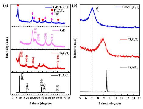
Fig. 4 (a) High angle and (b) low angle XRD patterns of  $Ti_3AlC_2$  powder,  $Ti_3C_2T_x$  MXene, mesoporous CdS nanoparticle, and the CdS/ $Ti_3C_2T_x$ heterostructure.
