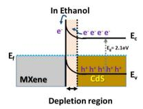
Fig. 8 The sensing mechanism of ethanol over the CdS/ $Ti_3C_2T_x$  composite
