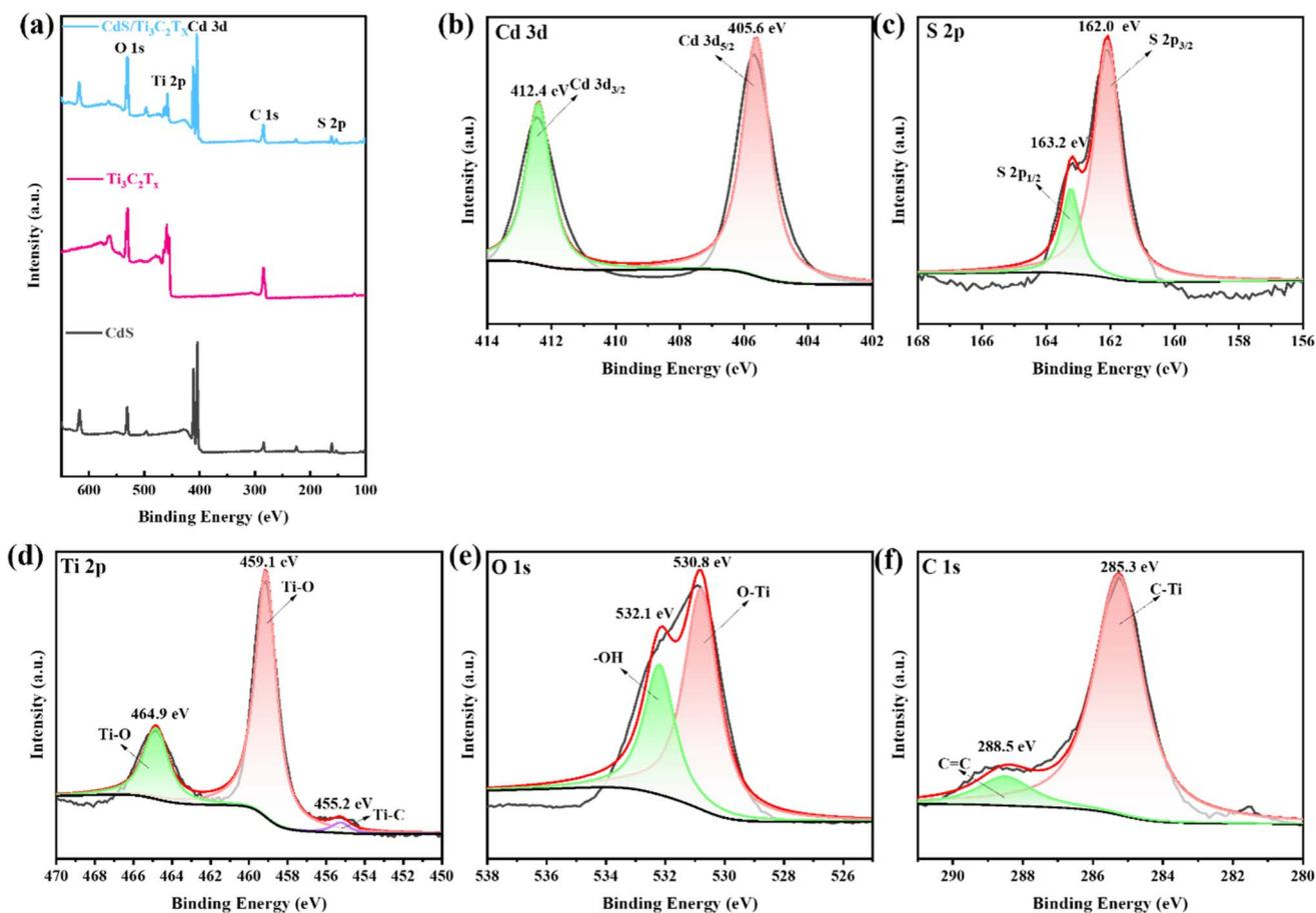
Fig. 5 (a) Survey spectra of the mesoporous CdS nanoparticle,  $\text{Ti}_3\text{C}_2\text{T}_x$  MXene, and CdS/ $\text{Ti}_3\text{C}_2\text{T}_x$  heterostructure. XPS spectra of the CdS/ $\text{Ti}_3\text{C}_2\text{T}_x$  heterostructure Cd 3d (b), S 2p (c), Ti 2p (d), O 1s (e), and C 1s (f).
