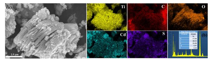
Fig. 3 (a) SEM images and (b) SEM-EDX elemental mapping of the CdS/ $Ti_3C_2T_x$  heterostructure.
