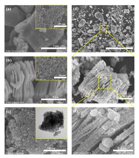
Fig. 2 SEM images of (a) pristine  $Ti_3AIC_2$ , (b)  $Ti_3C_2T_x$  MXene, (c) CdS (the inset figure is the TEM of CdS) and (d-f) the CdS/ $Ti_3C_2T_x$  heterostructure.
