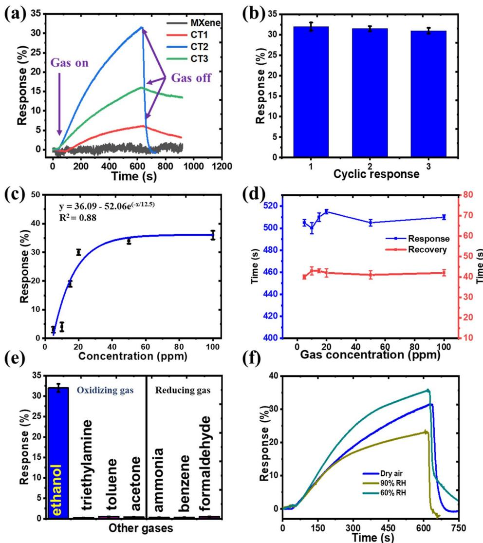
Fig. 7 (a) The response/recovery properties of pristine Ti<sub>3</sub>C<sub>2</sub>T<sub>x</sub> MXene, and prepared CdS/Ti<sub>3</sub>C<sub>2</sub>T<sub>x</sub>-based sensors, toward ethanol molecules (20 ppm). (b) Repeatability curve and (c) Langmuir isotherm curve of CT2 responses against different ethanol concentrations, and (d) response and recovery time. Response of the CT2 sensor to (e) several gases (f) at various levels of relative humidity.
