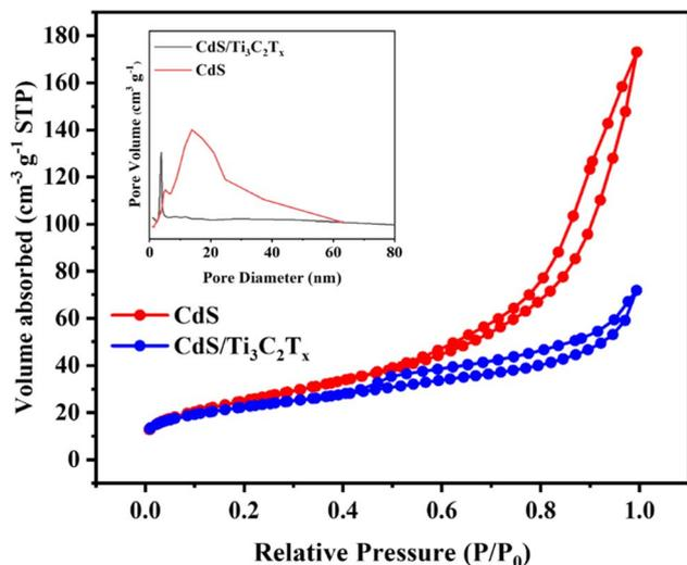
Fig. 6 Nitrogen adsorption-desorption isotherms were conducted for  $\text{Ti}_3\text{C}_2\text{T}_x$  MXene, mesoporous CdS nanoparticles, and the CdS/ $\text{Ti}_3\text{C}_2\text{T}_x$  heterostructure. Pore-size distributions are depicted in the inset.
