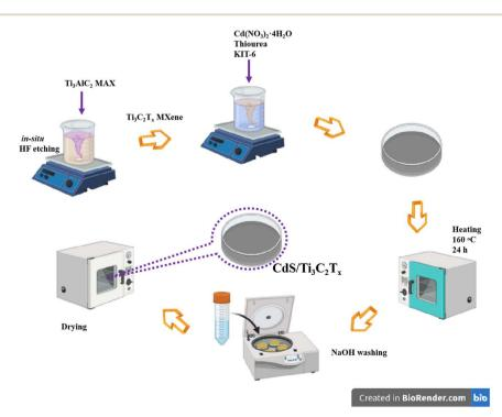
Fig. 1 Synthesis of CdS/Ti<sub>3</sub>C<sub>2</sub>T<sub>x</sub> composites (schematic).
