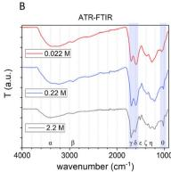
Fig. 3 Effect of the precursor concentration on the bulk structure of CNPs. (A) Normalized baseline-subtracted Raman spectra of CNPs synthesized starting from 0.022 M (red), 0.22 M (blue) and 2.2 M (grey) glucose aqueous solutions with a synthesis time of 3 h at 190 °C. (B) ATR-FTIR of the same samples (Greek letters refer to band assignation, see Table 3).
