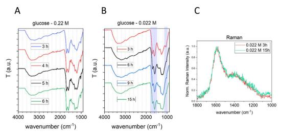
Fig. 4 Effect of the time of synthesis on the bulk structure of CNPs. (A and B) ATR-FTIR spectra of CNPs synthesized starting from 0.22 M (A) and 0.022 M (B) glucose at different synthesis times. (C) Normalized baseline-subtracted Raman spectra of CNPs synthesized in 3 h (red) and 15 h (green) starting from 0.022 M glucose.
