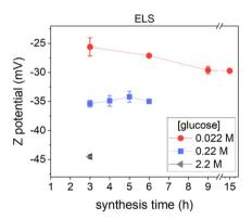
Fig. 2 Effect of the synthetic parameters on CNP ζ-potential. ζpotential of CNPs synthesized starting from 0.022 M (red circles), 0.22 M (blue squares) and 2.2 M glucose solutions (grey triangle) at the different synthesis times tested, all measured at pH  $\sim$ 4.
