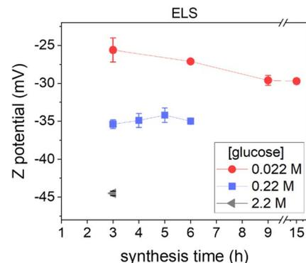
Fig. 2 Effect of the synthetic parameters on CNP  $\zeta$ -potential.  $\zeta$ -potential of CNPs synthesized starting from 0.022 M (red circles), 0.22 M (blue squares) and 2.2 M glucose solutions (grey triangle) at the different synthesis times tested, all measured at pH  $\sim 4$ .
