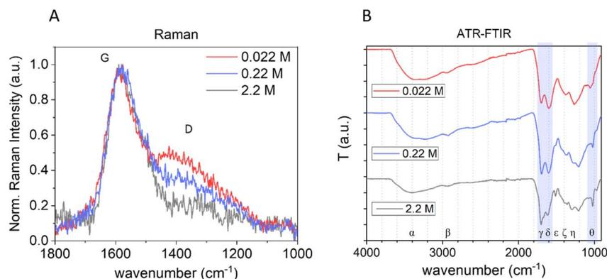
Fig. 3 Effect of the precursor concentration on the bulk structure of CNPs. (A) Normalized baseline-subtracted Raman spectra of CNPs synthesized starting from 0.022 M (red), 0.22 M (blue) and 2.2 M (grey) glucose aqueous solutions with a synthesis time of 3 h at 190 °C. (B) ATR-FTIR of the same samples (Greek letters refer to band assignment, see Table 3).
