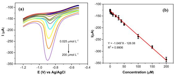
Fig. 12 (a) SWV curves of AgNPs@GO/IL@SPCE (E5) in 0.1 mol  $L^{-1}$  PBS (pH 7) containing different concentrations of MP (0.025–200  $\mu$ mol  $L^{-1}$ ); potential range (-0.5 to -1.2 V), amplitude 0.1 V; frequency 20 Hz. (b) The calibration plots of the peak currents vs. concentration of MP. Note: geometric area of the working electrode: 7 mm<sup>2</sup>.
