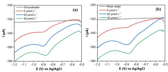
Fig. 14 (a) SWV curves of MP spiked with groundwater samples and (b) river water. Note: geometric area of the working electrode: 7 mm<sup>2</sup>.
