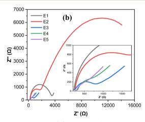
Fig. 6 (a) CV curves at a scan rate of 25 mV s<sup>-1</sup>, and (b) Nyquist plots of 5.0 mmol L<sup>-1</sup> [Fe(CN)6]<sup>3-/4-</sup> in 0.1 mol L<sup>-1</sup> KCl obtained with a bare SPCE (E1), GO@SPCE (E2), AgNPs@SPCE (E3), GO/IL@SPCE (E4), and AgNPs@GO/IL@SPCE (E5). Note: geometric area of the working electrode: 7 mm<sup>2</sup>.
