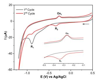
Fig. 8 Electrochemical behavior of MP (20  $\mu$ mol L<sup>-1</sup>; in 0.1 mol L<sup>-1</sup> PBS pH 7; scan rate 100 mV s $^{-1}$ ).
