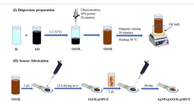
Fig. 1 Dispersion preparation (I) and sensor fabrication (II).
