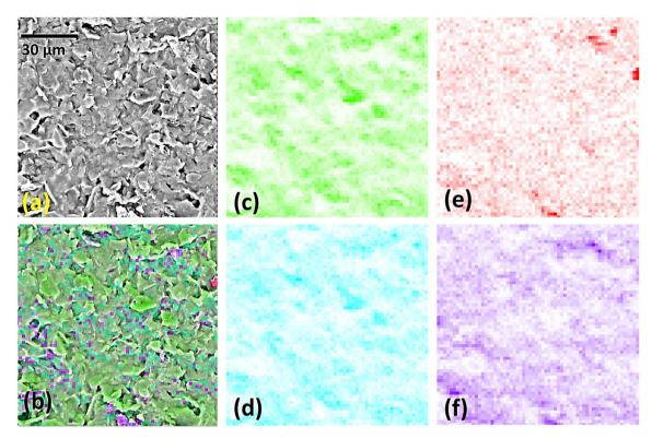
Fig. 5 AgNPs@GO/IL@SPCE electrode under the magnification of  $\times$ 2500 (a), full EDX map (b), and maps of selected elements: (c) carbon, (d) silver, (e) oxygen, and (f) fluorine. The analysis was done without Cu coating. The map resolution was 64  $\times$  64, limited by a relatively low conductivity of the electrodes without conductive coating, causing significant electron accumulation during the analysis.
