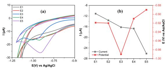
Fig. 10 (a) CVs of SPCE (E1), GO@SPCE (E2), AgNPs@SPCE (E3), GO/IL@SPCE (E4) and AgNPs@GO/IL@SPCE (E5) in the presence of 20  $\mu$ mol L<sup>-1</sup> MP in 0.1 mol L<sup>-1</sup> PBS (pH 7); scan rate 100 mV s<sup>-1</sup>. (b) The variation of  $I_{pa}$  and  $E_{pa}$  of MP reduction at different electrodes. Note: geometric area of the working electrode: 7 mm<sup>2</sup>.
