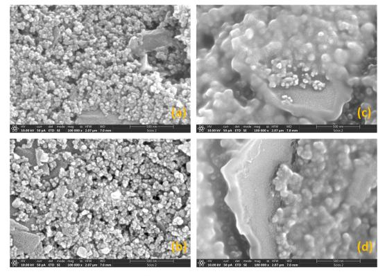
Fig. 4 High-resolution images (magnification ×100 000) of (a) GO@SPCE, (b) AgNPs@SPCE, (c) GO/IL@SPCE, and (d) AgNPs@GO/IL@SPCE sensor electrodes (recorded after covering the electrodes with a thin Au layer).
