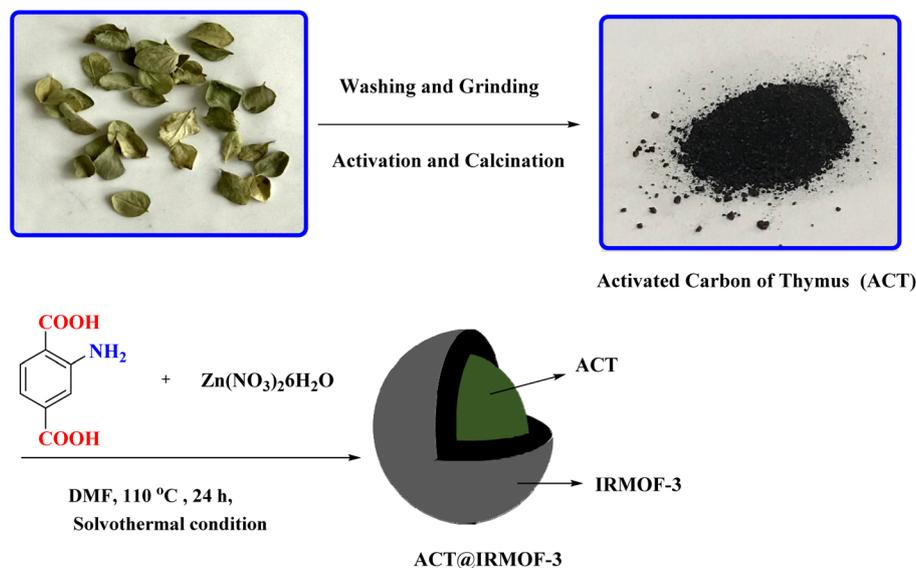
Fig. 2 The process of ACT@IRMOF-3 core-shell fabrication.
