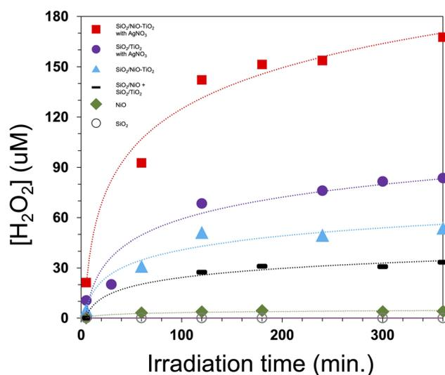
Fig. 3 Plot of  $[\text{H}_2\text{O}_2]$  vs. time under irradiation of aqueous suspension of catalyst. Legend: square =  $\text{SiO}_2/\text{NiO-TiO}_2$  w/  $\text{AgNO}_3$ ; circle =  $\text{SiO}_2/\text{TiO}_2$  w/  $\text{AgNO}_3$ ; triangle =  $\text{SiO}_2/\text{NiO-TiO}_2$ ; dash =  $\text{SiO}_2/\text{NiO} + \text{SiO}_2/\text{TiO}_2$ ; diamond = NiO; open circle =  $\text{SiO}_2$ .
