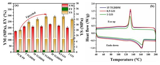
Fig. 3 (a) Mechanical properties of PCR PP vitrimers at room temperature and (b) the DSC thermogram illustrates the melting and crystallization behaviour of PCR PP vitrimers, both with and without nanofillers, emphasizing that the dynamic network has a trivial impact on the crystallization process of the vitrimers.
