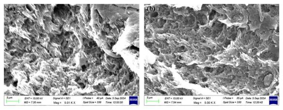
SEM micrograph of tensile fractured surfaces of (a) the PCR PP vitrimer (15 TGDDM) and (b) its nanocomposites (0.5 GO)
