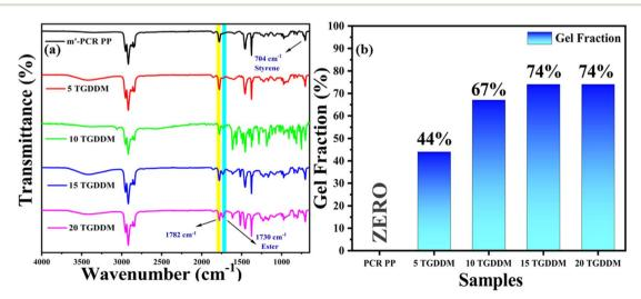
Fig. 2 (a) FT-IR spectrum of m'-PCR PP and vitrimers with different concentrations of TGDDM. (b) Gel fraction of PCR PP and PCR PP vitrimers.
