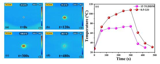
Fig. 6 (a-d) Infrared thermal image of the PCR PP vitrimer nanocomposite (0.5 GO) subjected to laser heating and (e) temperature vs. time graph upon heating and cooling for the PCR PP vitrimer (15 TGDDM) and its nanocomposite (0.5 GO).
