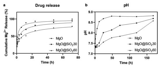
Fig. 4 (a) The released  ${\rm Mg^{2+}}$  fluctuation curve of MgO NPs, MgO@SiO\_30 and MgO@SiO\_60 nanocapsules (Mg<sup>2+</sup>, 5 mM) monitored by ICP-MS at different times in 10 mL deionized water. (b) The pH value fluctuation curve of MgO NPs, MgO@SiO\_30 and MgO@SiO\_60 nanocapsules monitored during immersing for 1 week in 10 mL deionized water.
