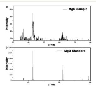
Fig. 1 (a) XRD pattern of the MgO NP sample. (b) XRD pattern of the MaO standard.
