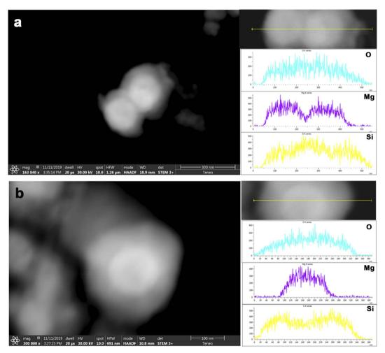
Fig. 3 (a) The shape and element composition of MgO@SiO $_2$ 30 nanocapsules using scanning transmission electron microscopy (STEM) and an energy dispersive spectrum (EDS). (b) The shape and element composition of MgO@SiO $_2$ 60 nanocapsules using STEM and EDS.
