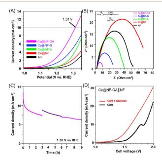
Fig. 4 LSV curves (A), Nyquist plots (the inset: a fitted equivalent circuit consisting of  $R_{\rm s}$ , CPE, and  $R_{\rm ct}$ ) (B) of the as-prepared samples and chronopotentiometry curves of Ce@NF-GA (C) and cell voltage comparison of glucose electrolysis and water electrolysis with Ce@NF-GA (D) at a scan rate of 5 mV s $^{-1}$ .
