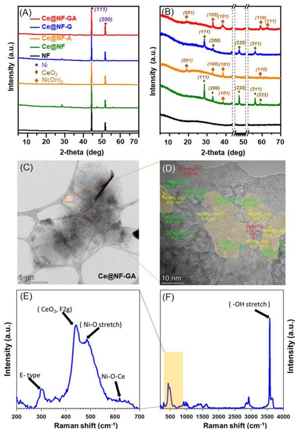
Fig. 2 XRD patterns (A), corresponding magnification of XRD patterns (B) of the as-prepared samples, TEM and HR-TEM image (C and D) and Raman spectra (E and F) of Ce@NF-GA.
