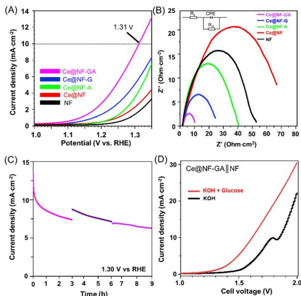
Fig. 4 LSV curves (A), Nyquist plots (the inset: a fitted equivalent circuit consisting of  $R_s$ , CPE, and  $R_{ct}$ ) (B) of the as-prepared samples and chronopotentiometry curves of Ce@NF-GA (C) and cell voltage comparison of glucose electrolysis and water electrolysis with Ce@NF-GA (D) at a scan rate of 5 mV s<sup>-1</sup>.
