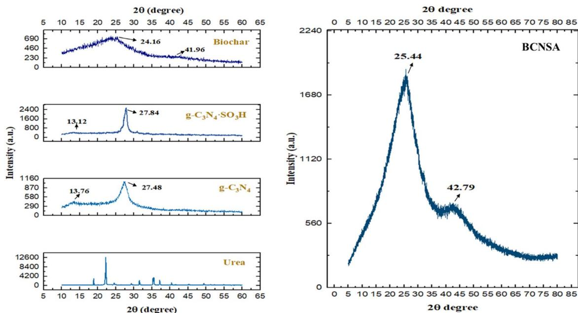
Fig. 3 The XRD graph of urea, g-C<sub>3</sub>N<sub>4</sub>, g-C<sub>3</sub>N<sub>4</sub>·SO<sub>3</sub>H, biochar and the synthesized BCNSA catalyst.
