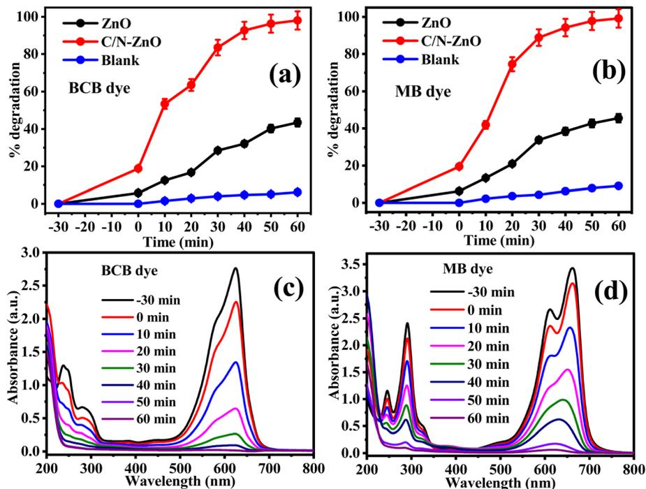
Fig. 8 Photodegradation performance of pure ZnO and C/N-co-doped-ZnO under visible light for (a) BCB (b) MB dyes, and UV-vis absorbance spectra for (c) BCB and (d) MB dyes in the presence of C/N-co-doped-ZnO under visible light.
