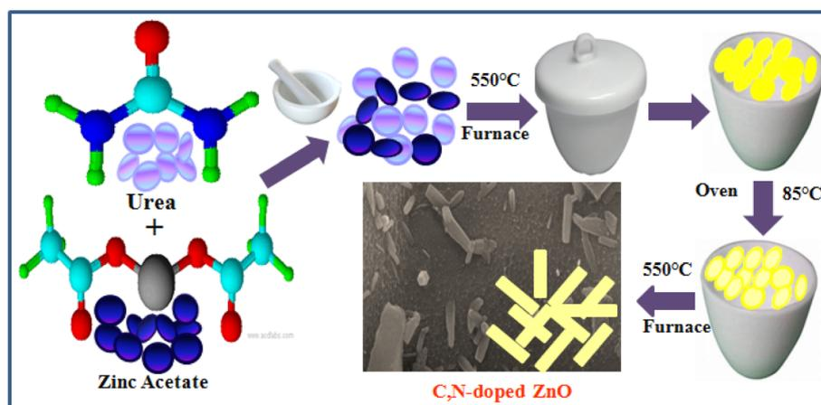
Fig. 1 Procedure for the synthesis of C/N-co-doped-ZnO nanorods.
